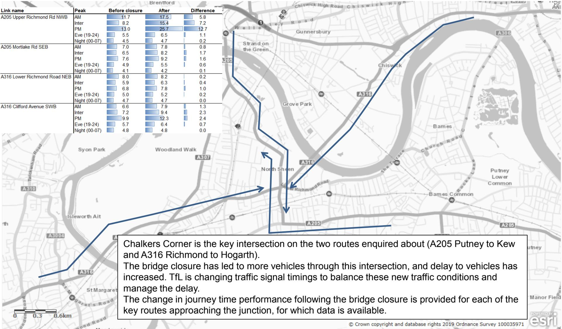
Chalkers Corner is the key intersection on the two routes enquired about (A205 Putney to Kew and A316 Richmond to Hogarth). The bridge closure has led to more vehicles through this intersection, and delay to vehicles has increased. TfL is changing traffic signal timings to balance these new traffic conditions and manage the delay. The change in journey time performance following the bridge closure is provided for each of the key routes approaching the junction, for which data is available.
