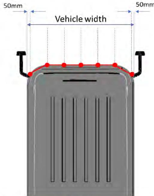
**Figure 15\_3: Virtual profile for determining impact for VUT**
