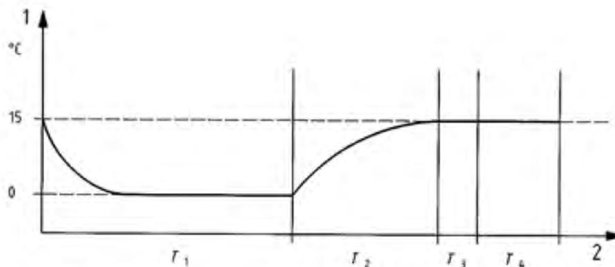
Figure 9\_1 – Zero emission bus heating test time profile
