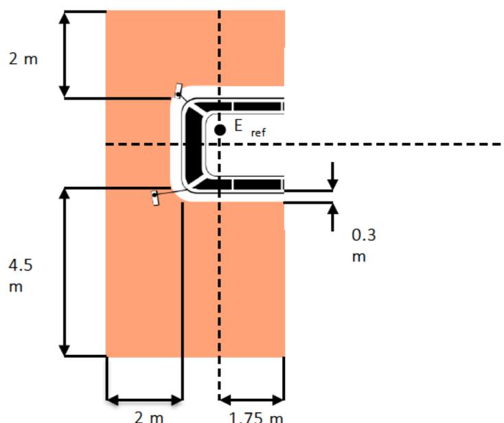
**Figure 19\_8: Plan view of forward close proximity assessment zone**
