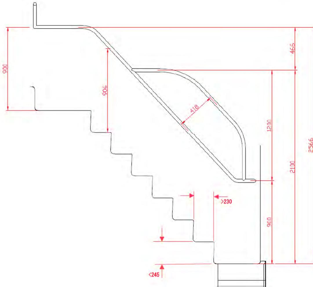
Figure 8\_1 Staircase handrail dimensions given in mm
