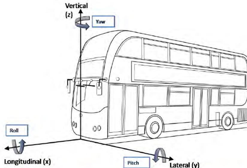
**Figure 24\_3: Local coordinate system and notation for VUT**
