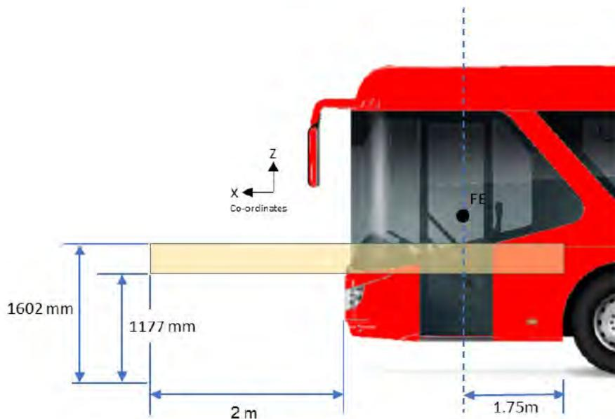
**Figure 19\_10: Side view of forward close proximity assessment zone**
