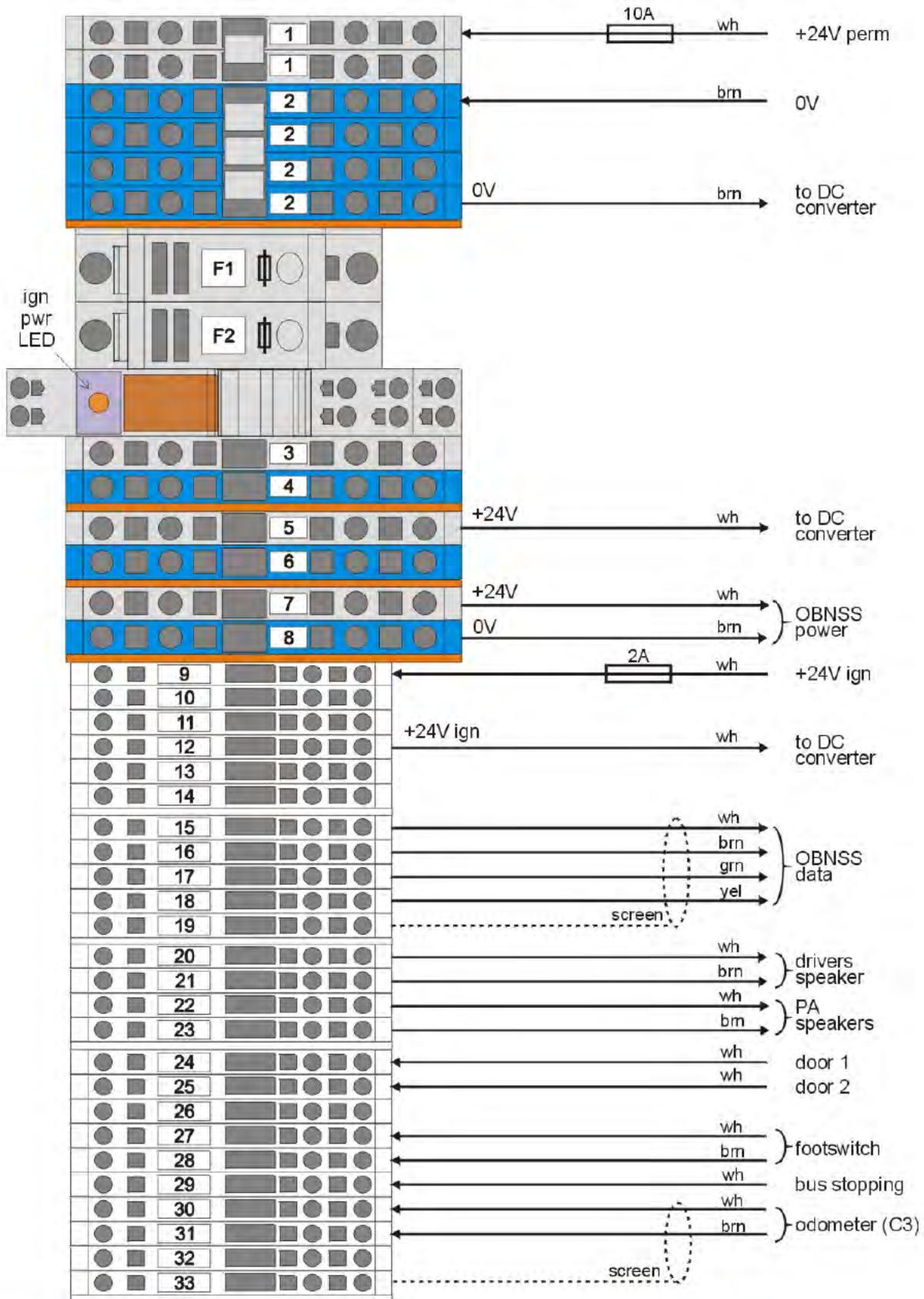
Figure 14\_5 iBus connection block external connection pin-outs
