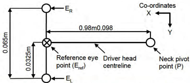
**Figure 19\_3: Definition of left and right eye point (E<sub>L</sub> and E<sub>R</sub>) positions relative to the neck pivot point (P) and reference eye point (E<sub>ref</sub>)**
