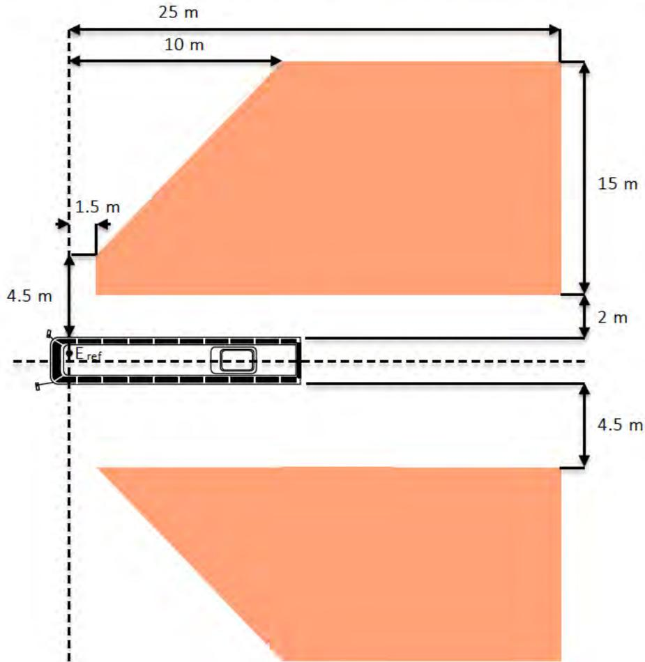
Figure 19\_13: Plan view of wide-angle assessment zone
