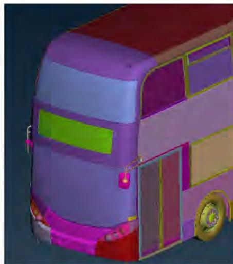
**Figure 19\_15: Example CAD data required for bus vision standard assessment**
