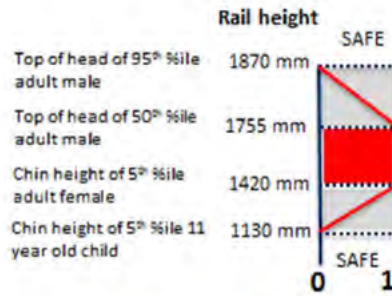
Figure 34_11: Illustration of assessment for horizontal handrail based on its height above the bus floor.
