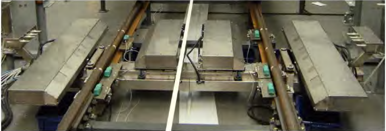
Figure 1 – AVIS wheel profile measurement system
