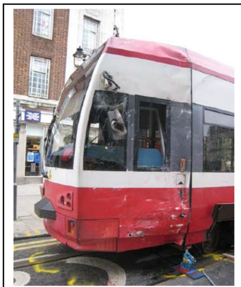
Damage to carriage of tram
