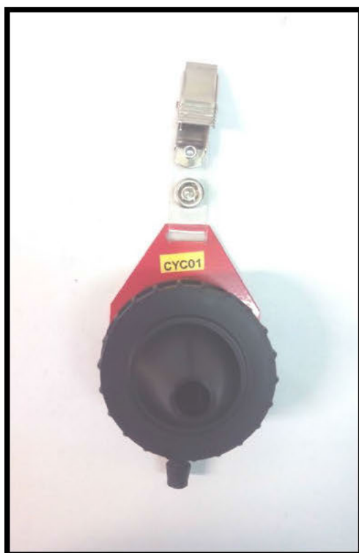
Figure 10. Cyclone Inhalable Sampler to monitor PM 2.5.
