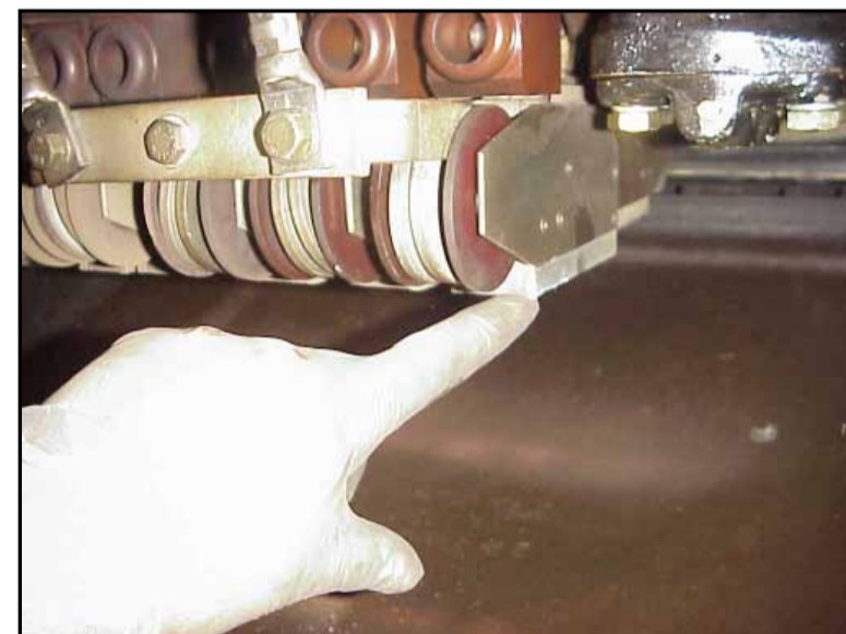
Incase No 2, outside of car, on side of train 7535 Flash guards Chrysotile
