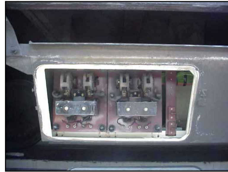
In screen megger points box, outside of car on side of train 17534 Flash guards Chrysotile
