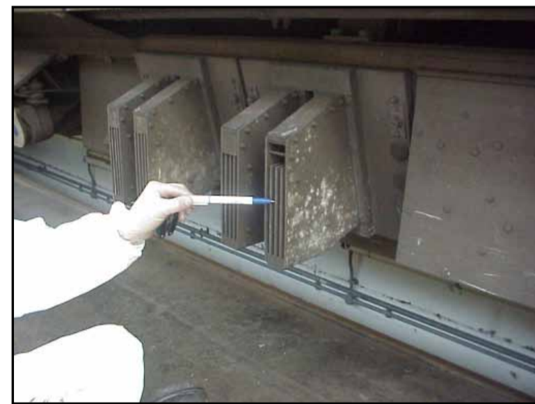
In equipment case No 10, outside car on side of the train Flash guards Chrysotile
