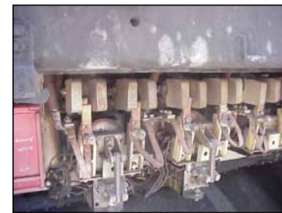
In equipment case No 1, outside car on the side of train 7534 Flash guards Chrysotile
