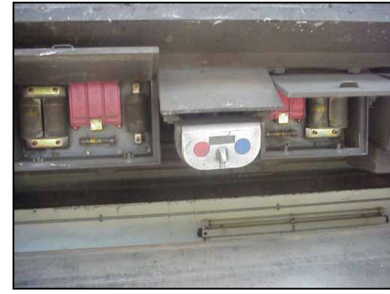
In fuse boxes linings, outside car on side of train 7535 Board. Chrysotile
