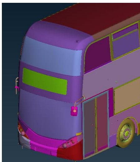
Figure 19_15: Example CAD data required for bus vision standard assessment
