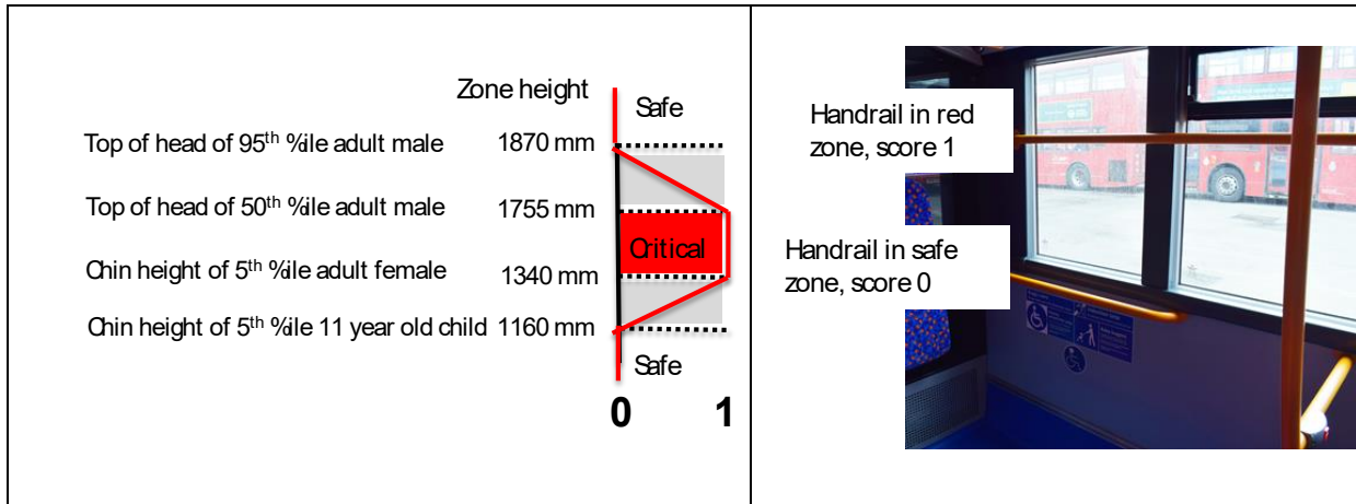
Figure 34_18: Illustration of assessment for horizontal handrails based on their height above the bus floor.
