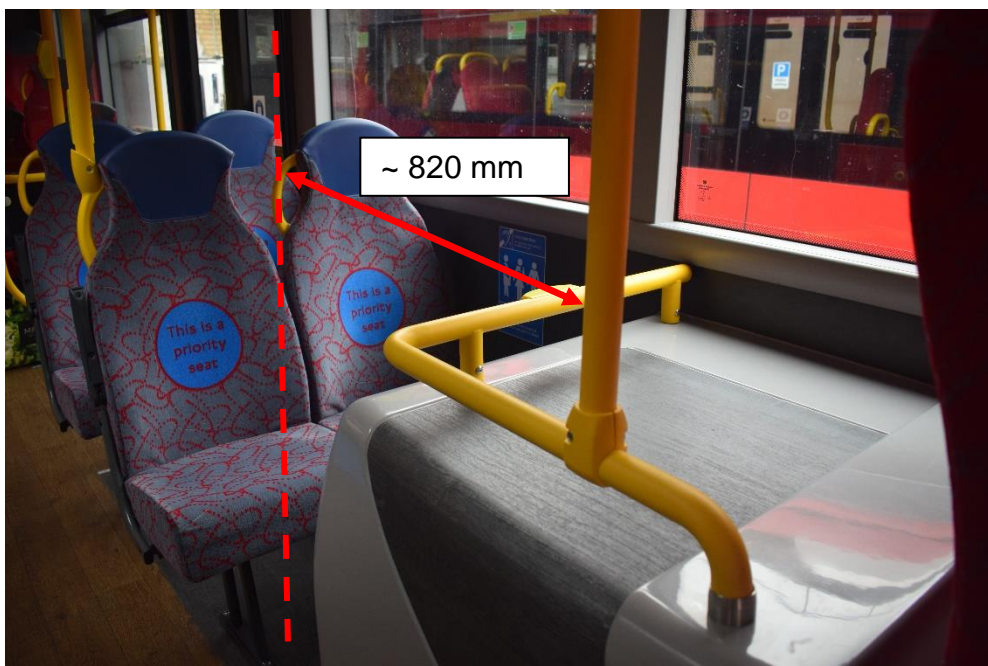
Figure 34_13: Assessment of vertical handrail positioned in front of seats behind luggage rack showing handrail > 750 mm longitudinally from front of seat cushion and therefore outside 'vertical handrail impact assessment zone'
