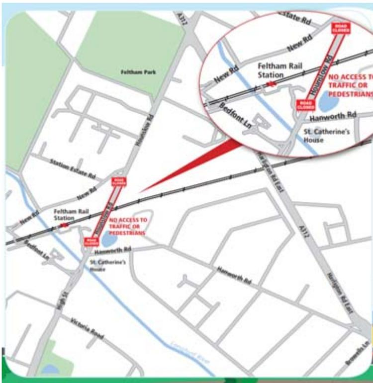
Phase 1 of the works involved the use of two sets of temporary traffic signals, at the existing priority-controlled junction of New Road/Hounslow Road, and the existing signalised junction of Hounslow Road/Hanworth Road/Station Approach/Bedfont Lane/High Street (25/133), as per the TM drawings attached.
