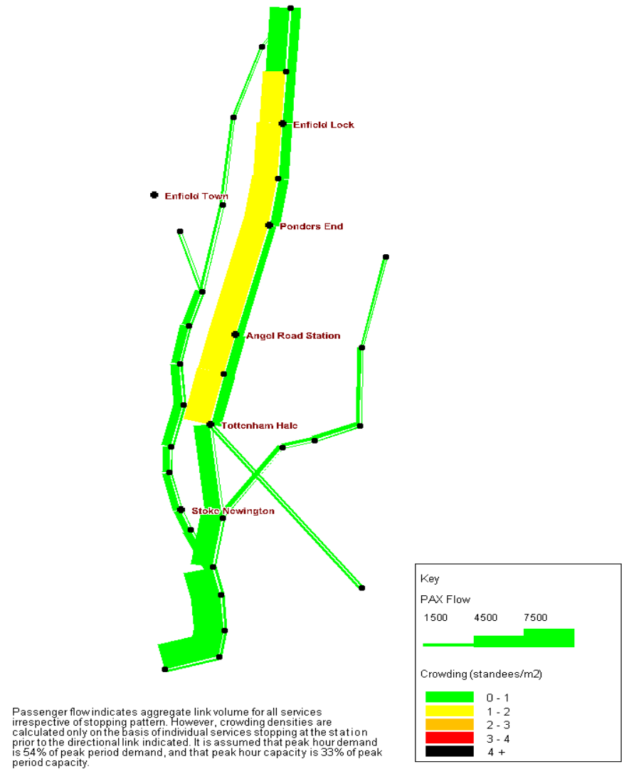
Figure 46 - NR Crowding and Flow, PM peak hour, 2021 ULV2 (growth and additional PT and mode shift interventions)
