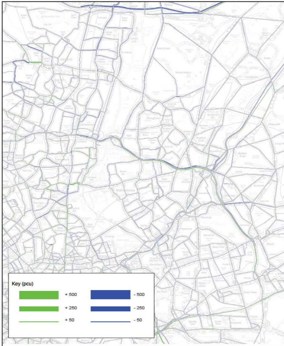
Figure 53 - Flow differences (pcu), AM peak hour, 2021 ULV1(growth and no interventions) – 2021 ULV2(growth and PT and mode shift interventions)
