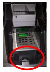
Last year we trialled an alternative design of block, initially on devices at Charing Cross, Green Park and Piccadilly Circus, using screws rather than adhesive to secure the PED block in place. As a result these blocks have a couple of small bumps in the top to cover these fixings.
