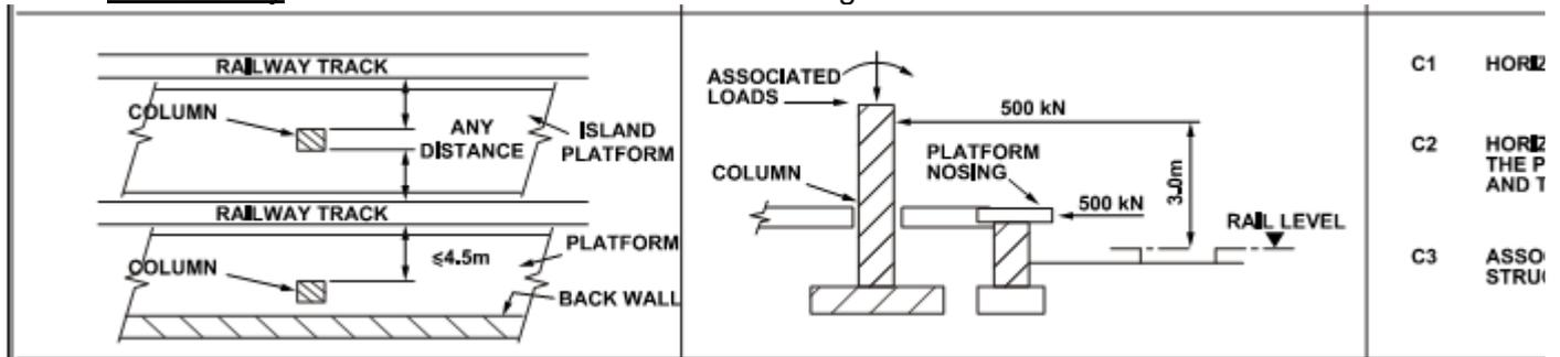
2. In areas where rail-road vehicles can circulate (see attached RSH&P sketch 11460\_SK\_0016) – do columns need to be designed for errant road vehicle protection loading as per paragraph [3.2.16.9](#) in TFL document S1053?
