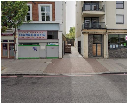
7. Uncontrolled crossing south of Elmfield Road junction. Traffic cylinder positioned in the middle of the crossing carpet presents a hazard to visually impaired / mobility impaired pedestrians and may result in trips/falls or users becoming stranded in the carriageway.
