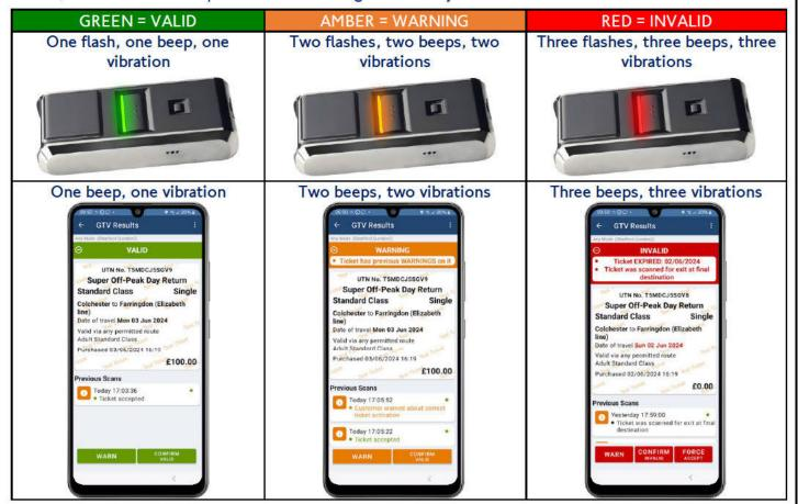
If an invalid ticket is scanned a red aspect will be shown on the reader and a claxon type rejection tone is sounded to highlight that the ticket is not valid.
