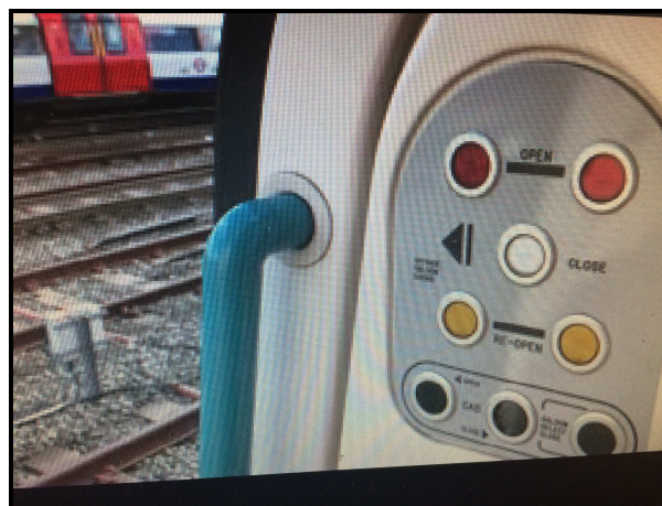
Figure 5– Image of DCIVs with saloon doors closed on a sunny day
