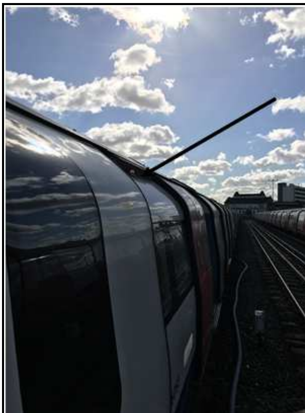
Figure 6 - Physical view of ODILs from driving side cab door
