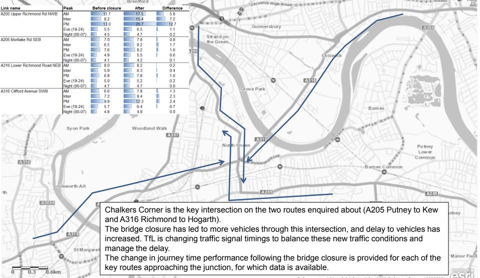
Average changes in weekday bus journey times (in minutes per km), between 07:00 and 19:00, since the bridge closure, with section journey times changes (in minutes) at key bottlenecks highlighted, based on iBus data (comparing 29<sup>th</sup> April to 5<sup>th</sup> July 2019 with the equivalent period in 2018)
