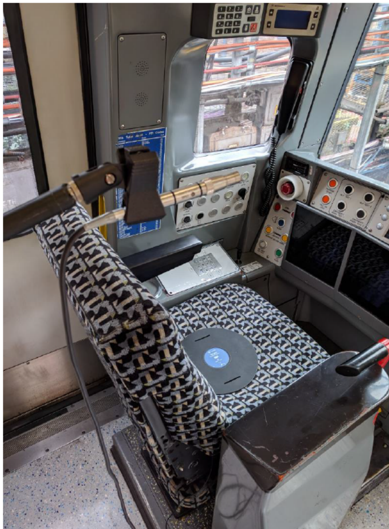
Figure C1 - Northern line 1995 tube stock cab and microphone arrangement
