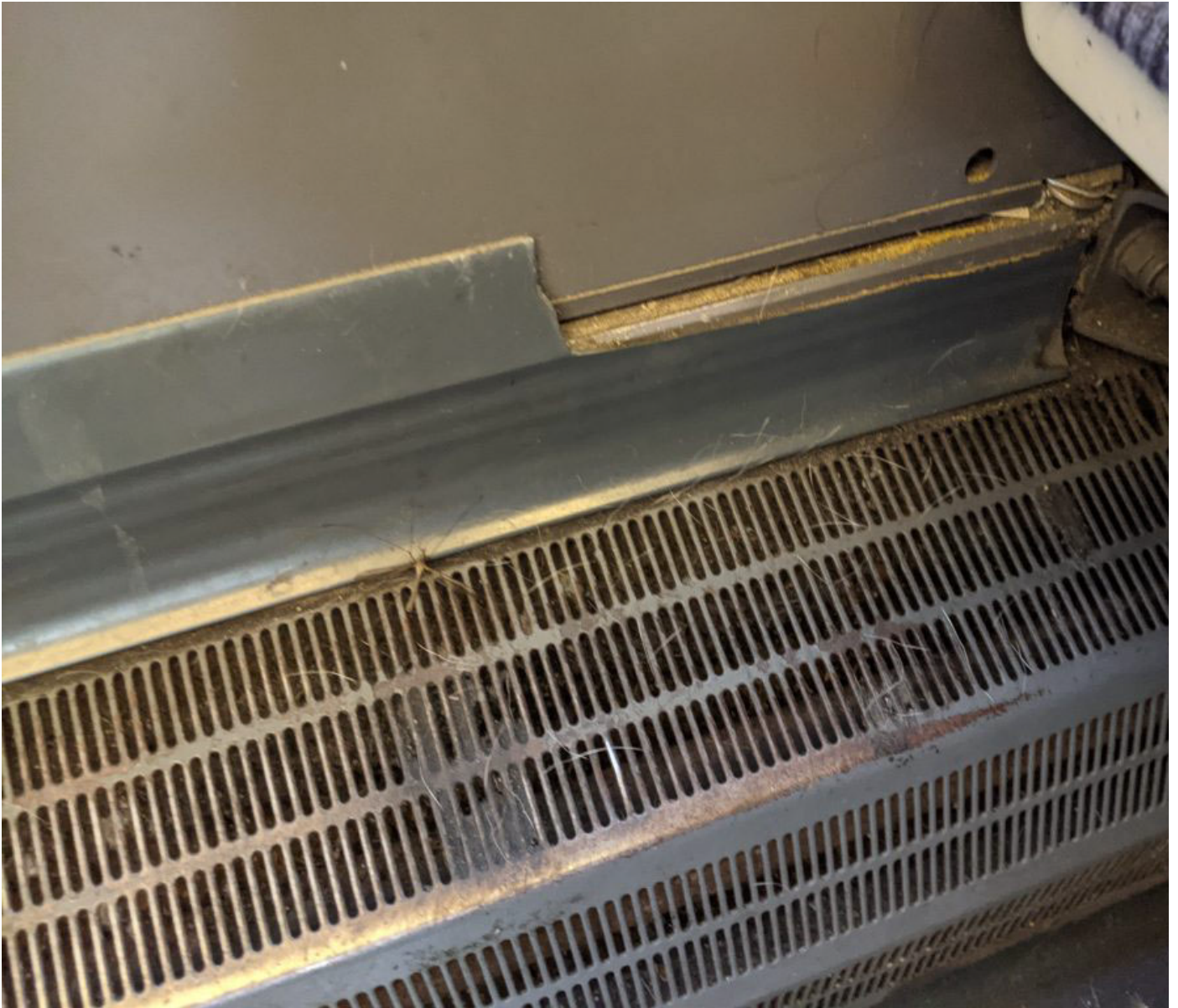
Filthy trains with various fittings loose or missing
