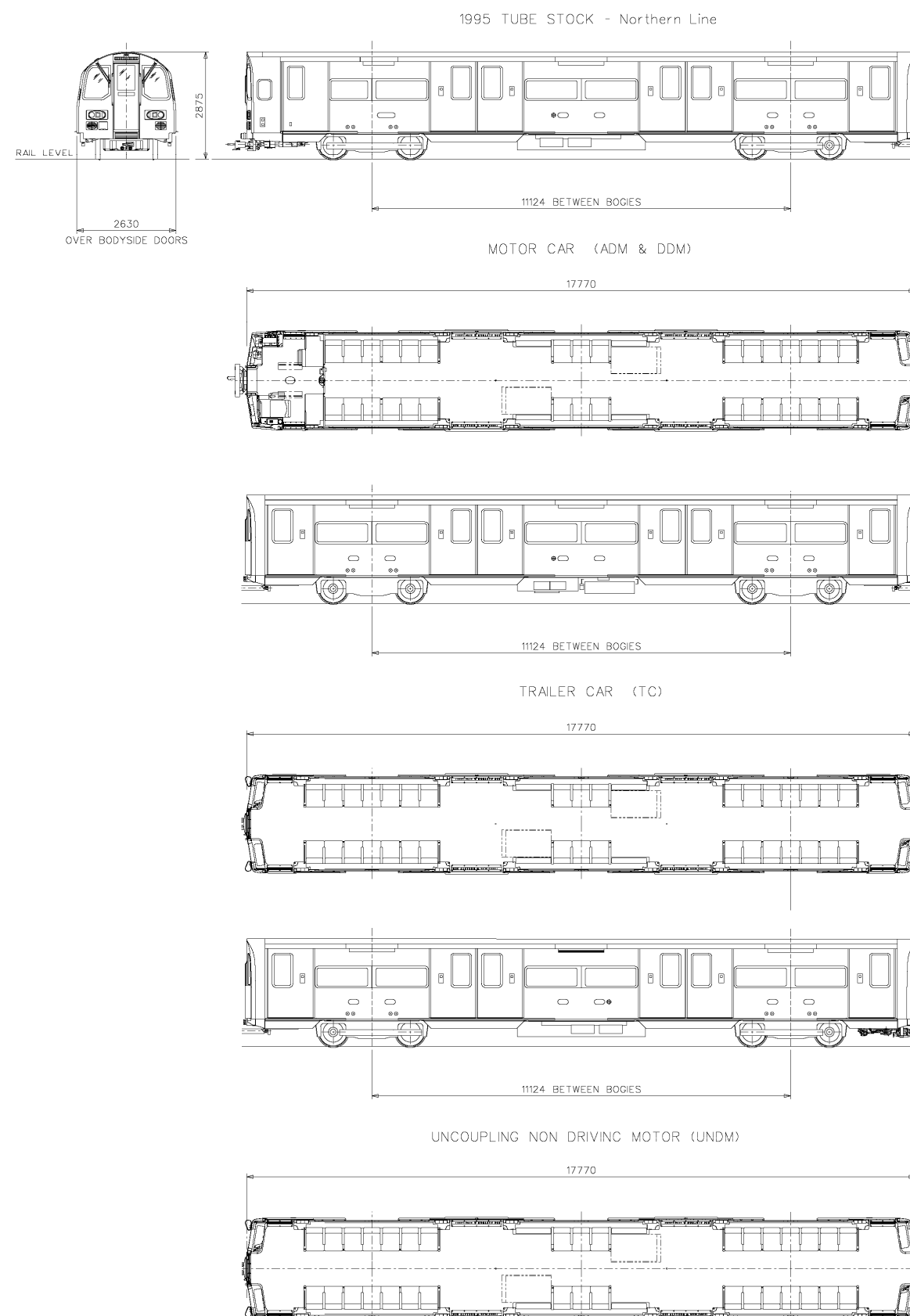
1995 TUBE STOCK - TARE WEIGHT - 156.66 TONNES - 6 CAR TRAIN
