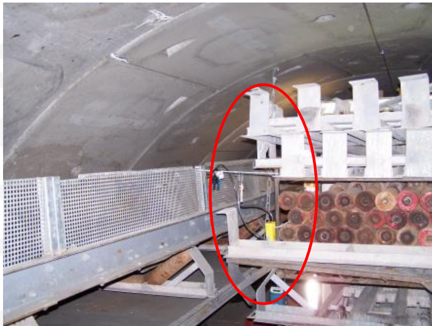
Figure 7: Static samplers located at conveyor extension area
