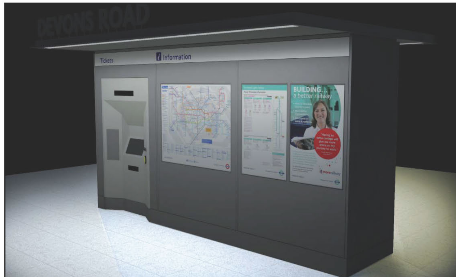
Lighting is integrated into the ticket machine modules providing a good level of illumination on the vertical surfaces displaying information. The light level is also increased noticeably at ground level to provide a horizontal marker for the presence of a task area.
