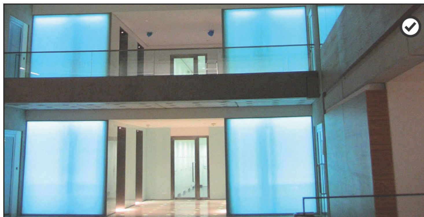
Illumination of opaque glass lifts acts both to draw attention to the lift locations for wayfinding and orientation and also as a decorative feature.
