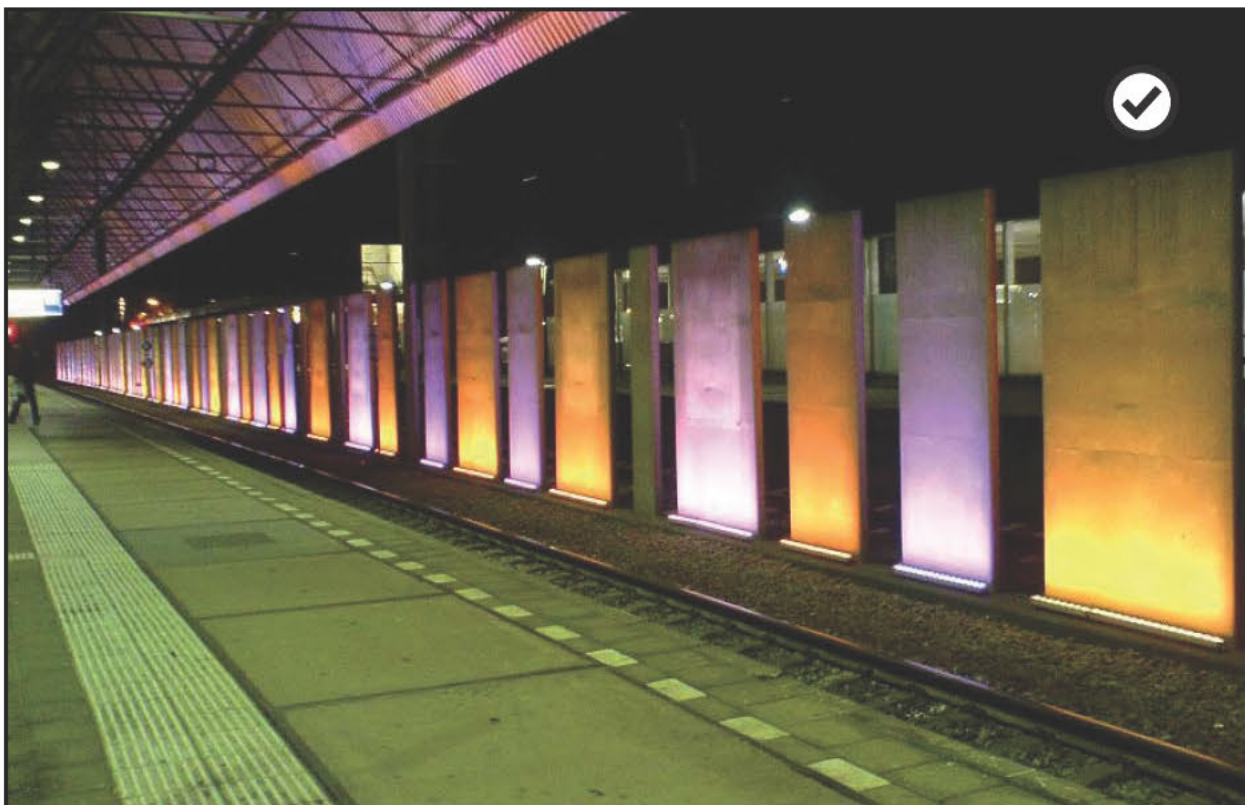
Up lighting and indirect light from the canopy form a distinct station identity.
