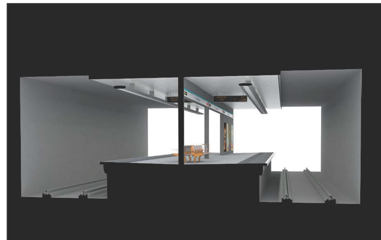
Underground Island Platform Layout – Layout is similar to the Island Platform layout.
