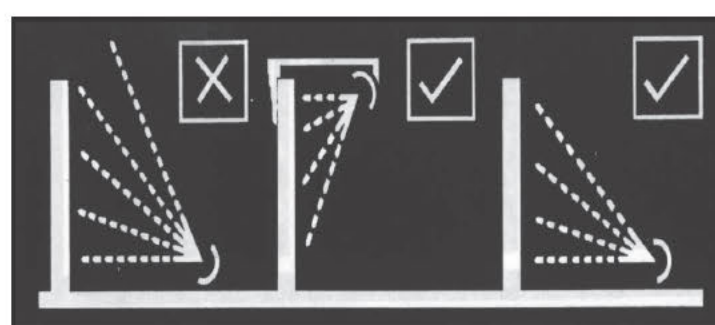
Ensuring good light out off angles
