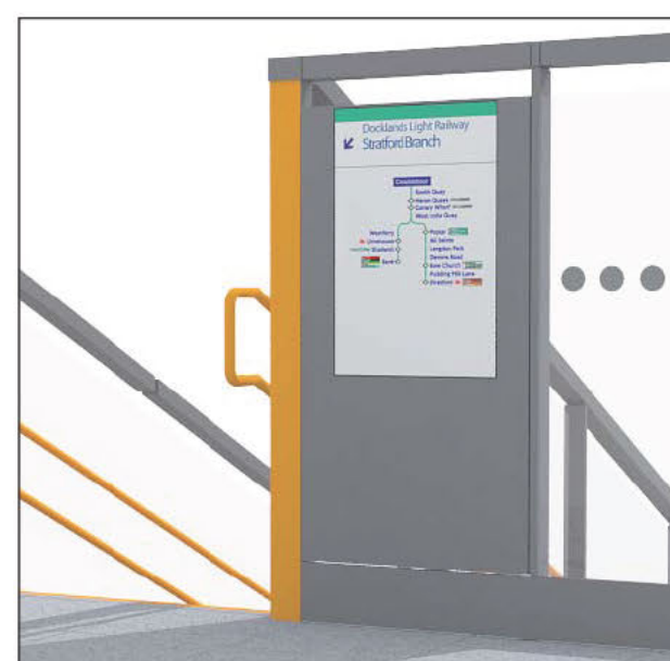
Screen/cladding mounted signs are used beside routes to platforms
