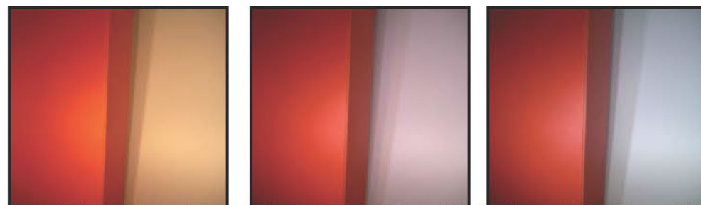
Example of colour temperature interaction on the same surface. Note the difference in the vibrancy of the red colour between the Warm (left) and Cool (right).
