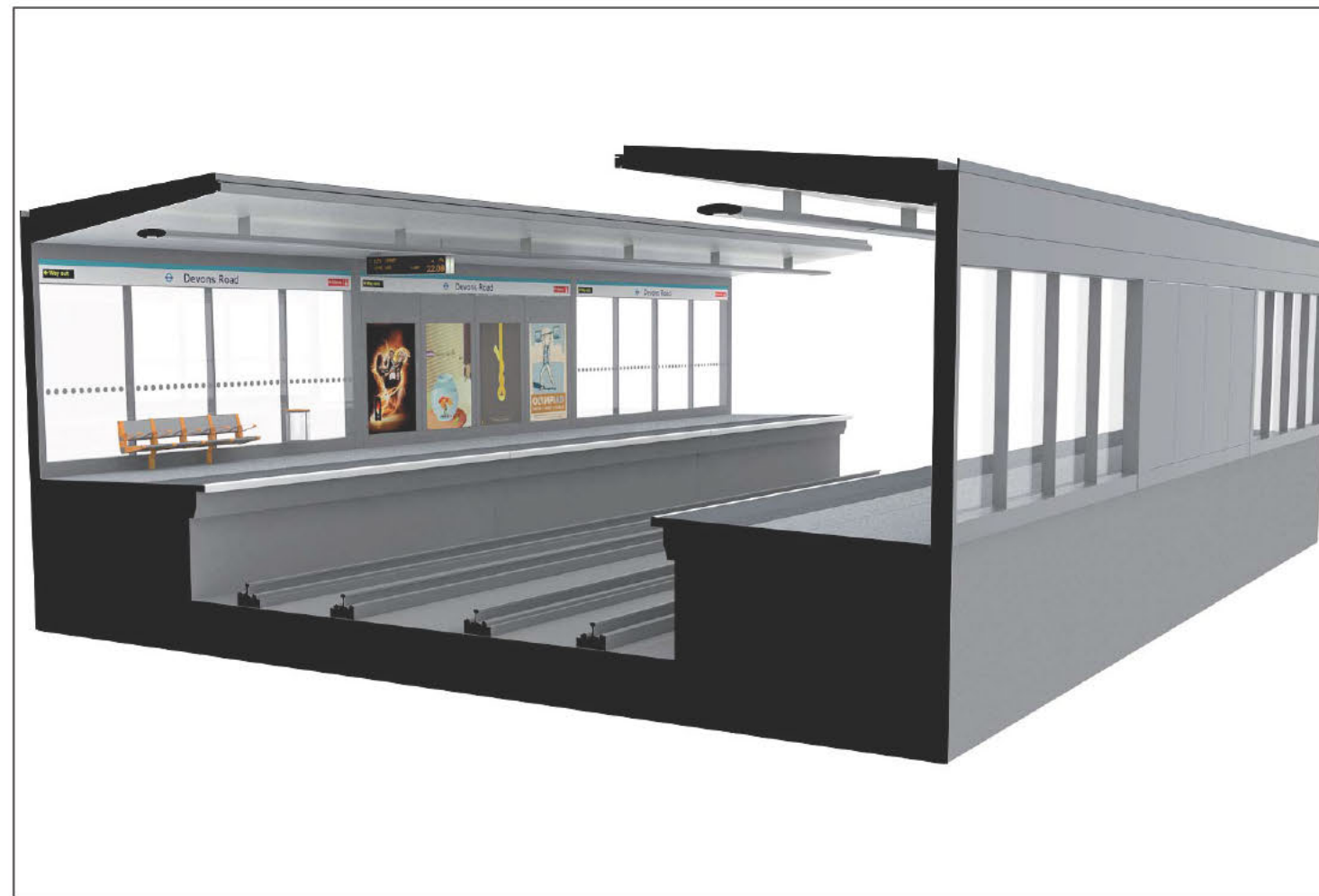
Side Platform Layout – where the platform is visible from the rear, the exterior surfaces should be flush as well. Other typologies are shown opposite.
