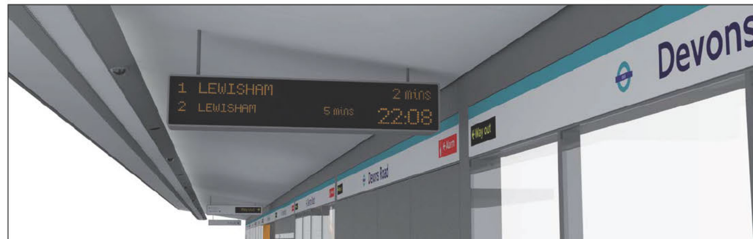
Platform Overhead Signage spacing permits visibility of signs and PIDs from 30m.
