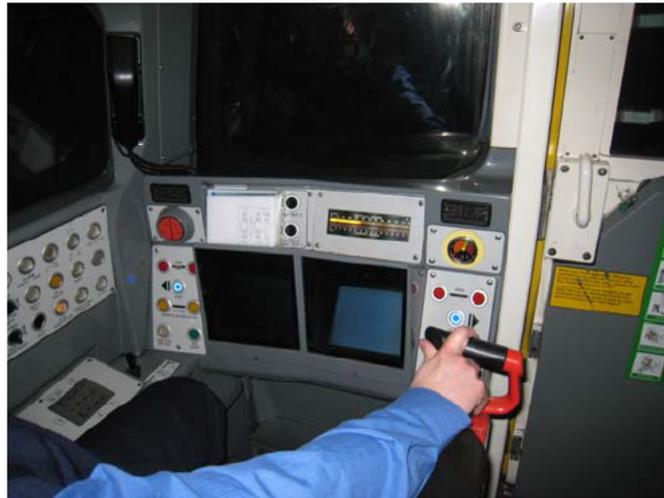
**Figure 4:** Examples of the use of key visual tasks that involve colour within the cabin. Information to the train driver is provided by means of displays and other controls that differ in size, shape, position, colour and luminance. Intermittent lights and audible signals are also used.
