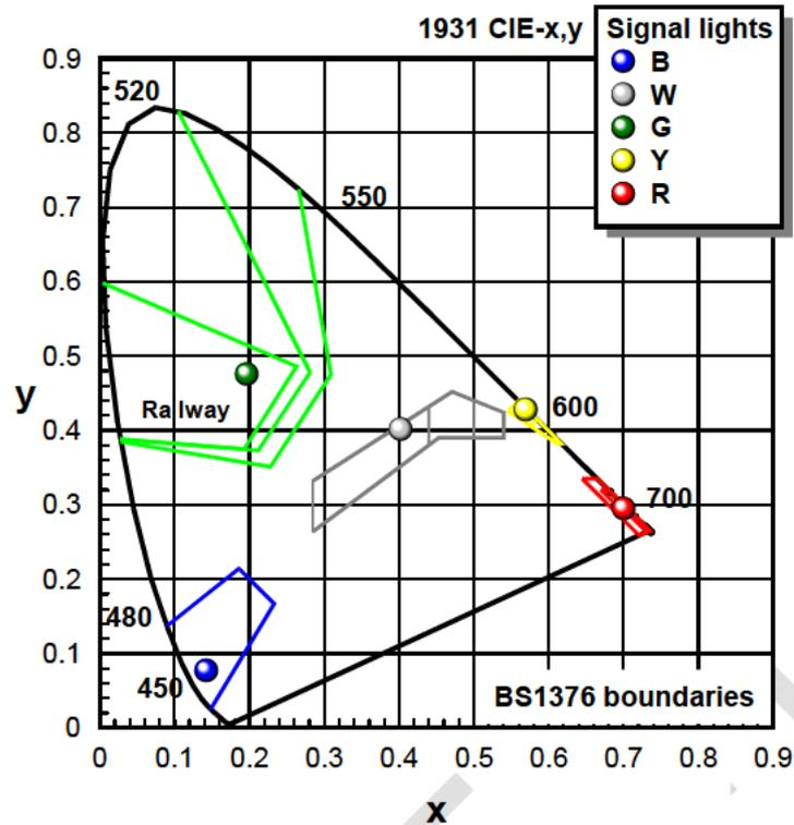
**Figure 18:** 1931 CIE-x,y colour space diagram showing the recommended chromaticity boundaries for the colours of light signals (BS 1376, 1974; CIE, 2001). The coloured discs plot the signal colours reproduced in the laboratory.
