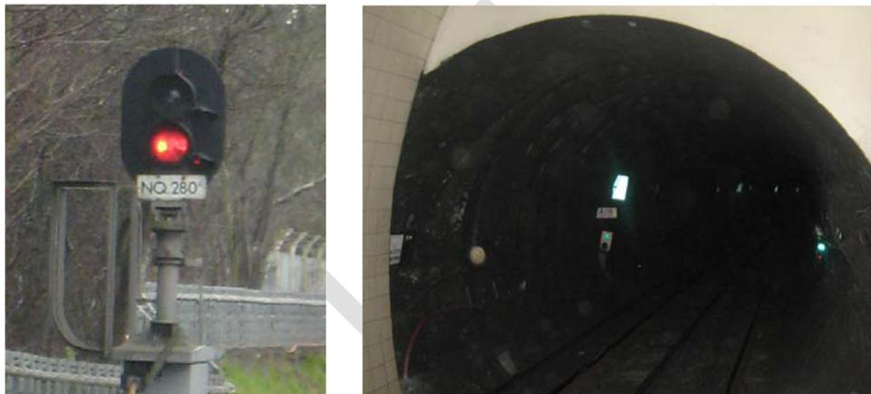
**Figure 1:** (a) Open air track-red signal light. The red signal lights are always positioned on the bottom of the two aspect signal house to correspond to the driver's line of sight. (b) St. John Wood station: Co-acting signal, i.e. a signal on both sides of the tunnel. It has been reported that the installation of the co-acting signal has reduced the number of SPADs at this station.
