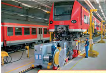
An Example of a Mobile Wheel Lathe in a non- London Underground Depot
