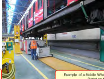
Example of a Mobile Wheel Lathe in operation at Ruislip Depot on the Central Line
