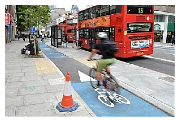
Bus stop bypasses allow a cycle lane to pass behind a bus shelter. They do this by creating a bus stop island, meaning that pedestrians must cross the cycle way to board a bus and when alighting a bus.
