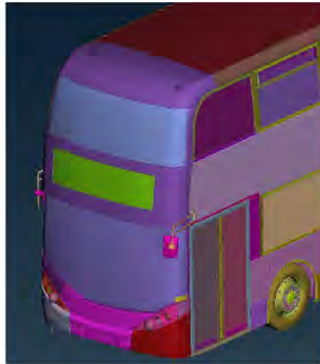
Figure 26: Example CAD data required for bus vision standard assessment
