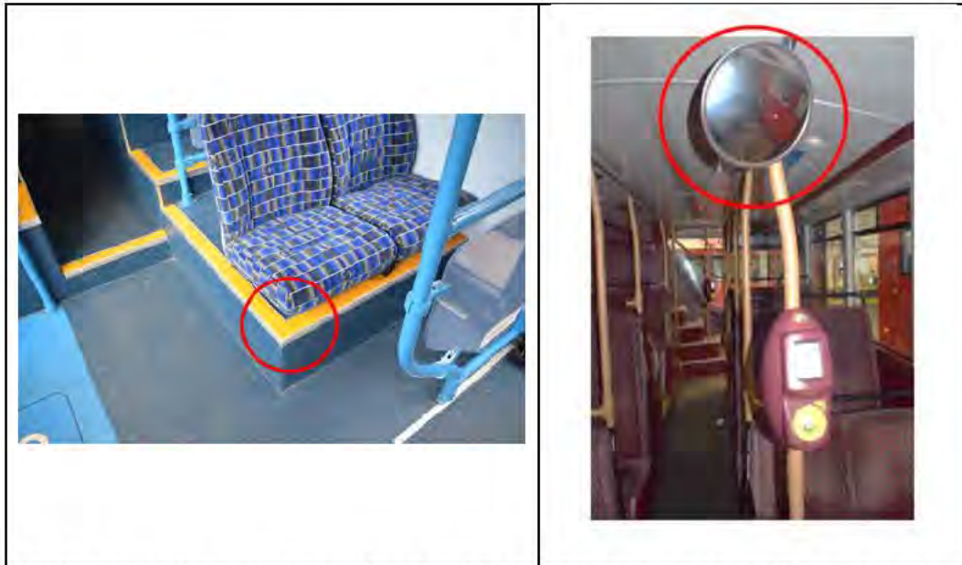
Figure 7: Examples of general hazards for standing passengers, corner of step (left) and mirror in head impact zone (right).
