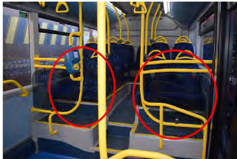
Figure 1: Examples of seats with high occupancy rate immediately adjacent to a door and only accessible via a step.
