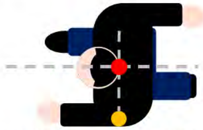
Figure 4: Origin of local coordinate systems for EPTa and EPTc test targets, illustrating test target hip point (orange), centrelines (grey) and local coordinate system origin (red)
