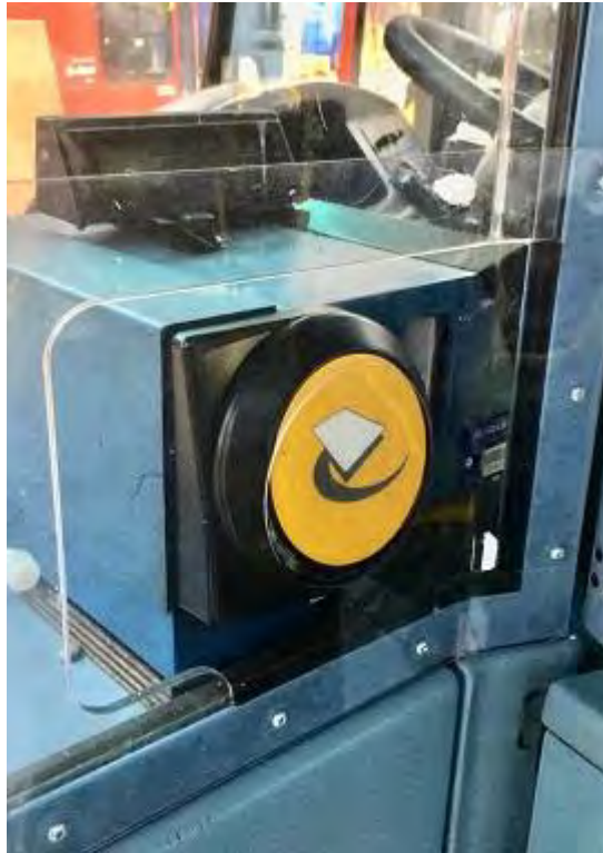
Figure 6_2: Flexible plastic over the top of Smart Card Reader pad. Held in place by a removable polycarbonate panel
