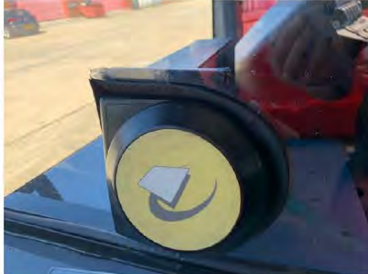
Figure 6_1: Smart Card Reader ONLY protrudes through the assault screen
