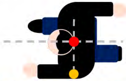
Figure 24_4: Origin of local coordinate systems for EPTa and EPTc test targets, illustrating centrelines (grey), local coordinate system origin (red) and test target hip point (orange),
