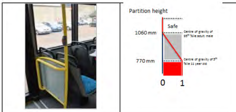
Figure 34_12: Illustration of assessment of restraint (partitions) for standing passengers.
