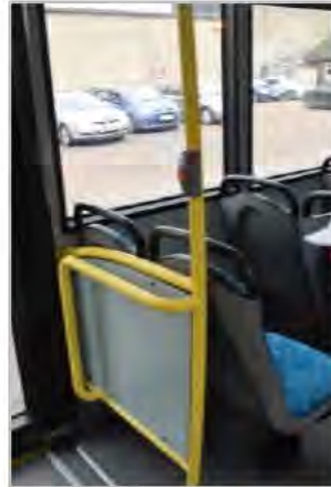
Figure 34_6: Example of partition consisting of multiple structures
