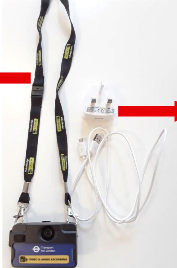
A wall charger and micro USB charging cable will be supplied. The video device can be charged via wall socket or a computer hard drive.
