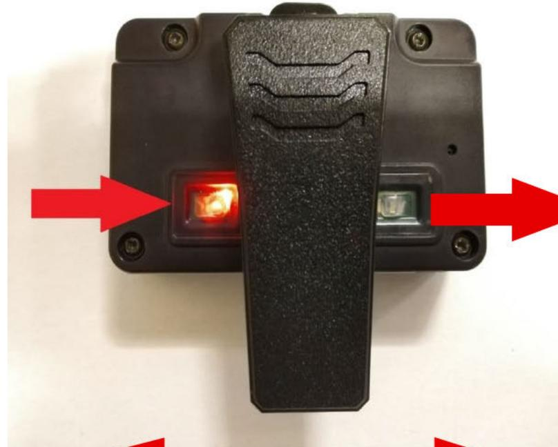
Activation button on either side – illuminates red when pressed
