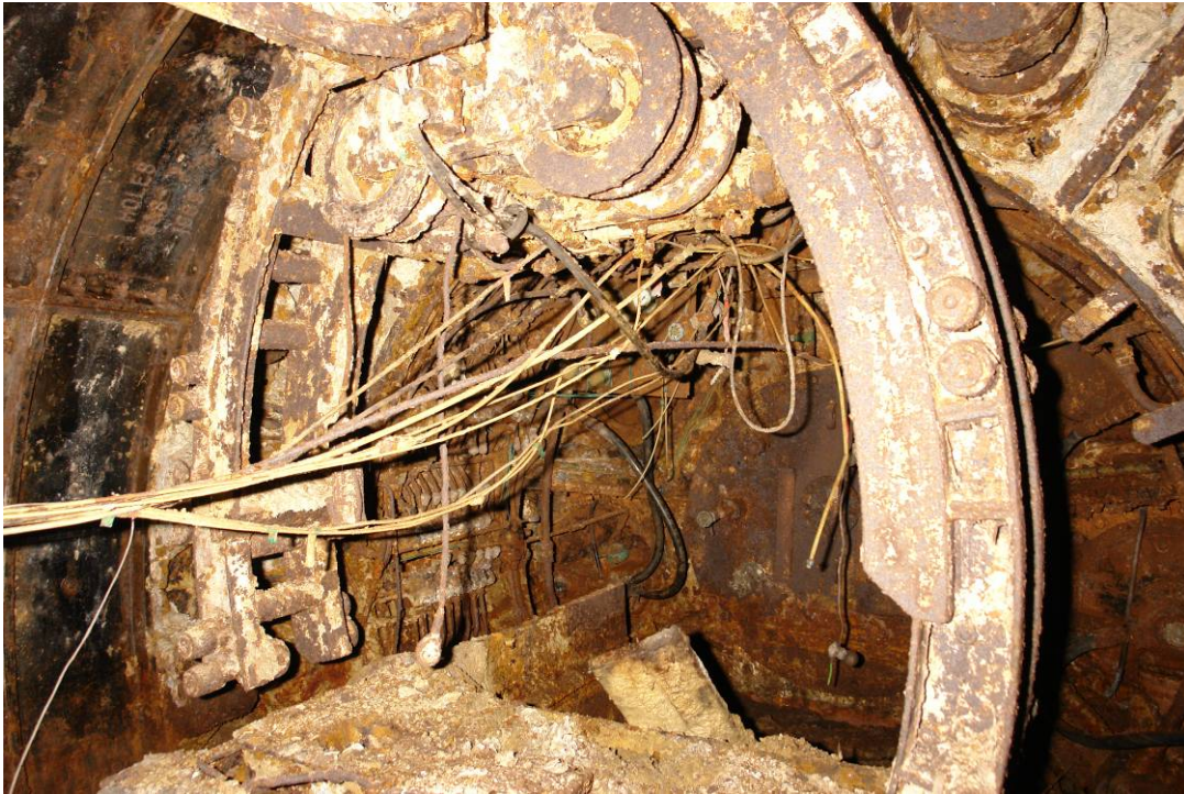
Figure 19 Pressure bulkhead of tunnelling machine retaining end face of tunnel
