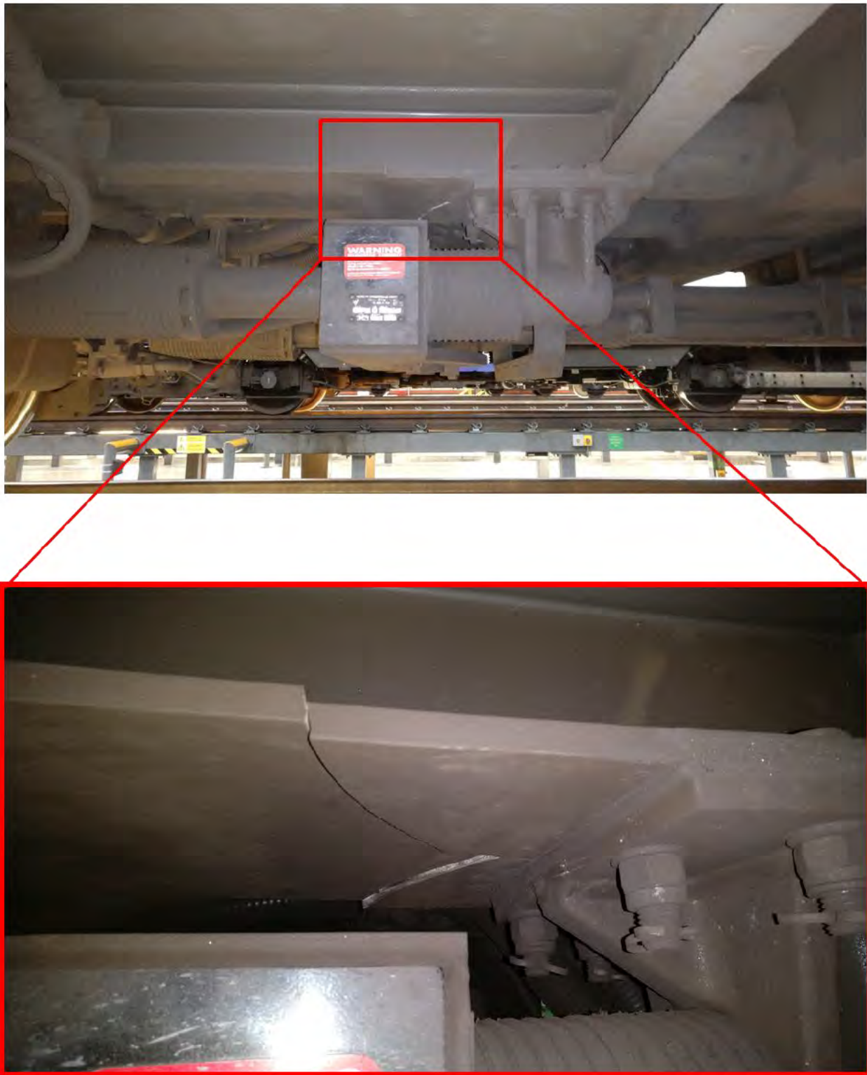
Figure 6: Image of car 96609 D End No. 2 side longitudinal beam fractures
