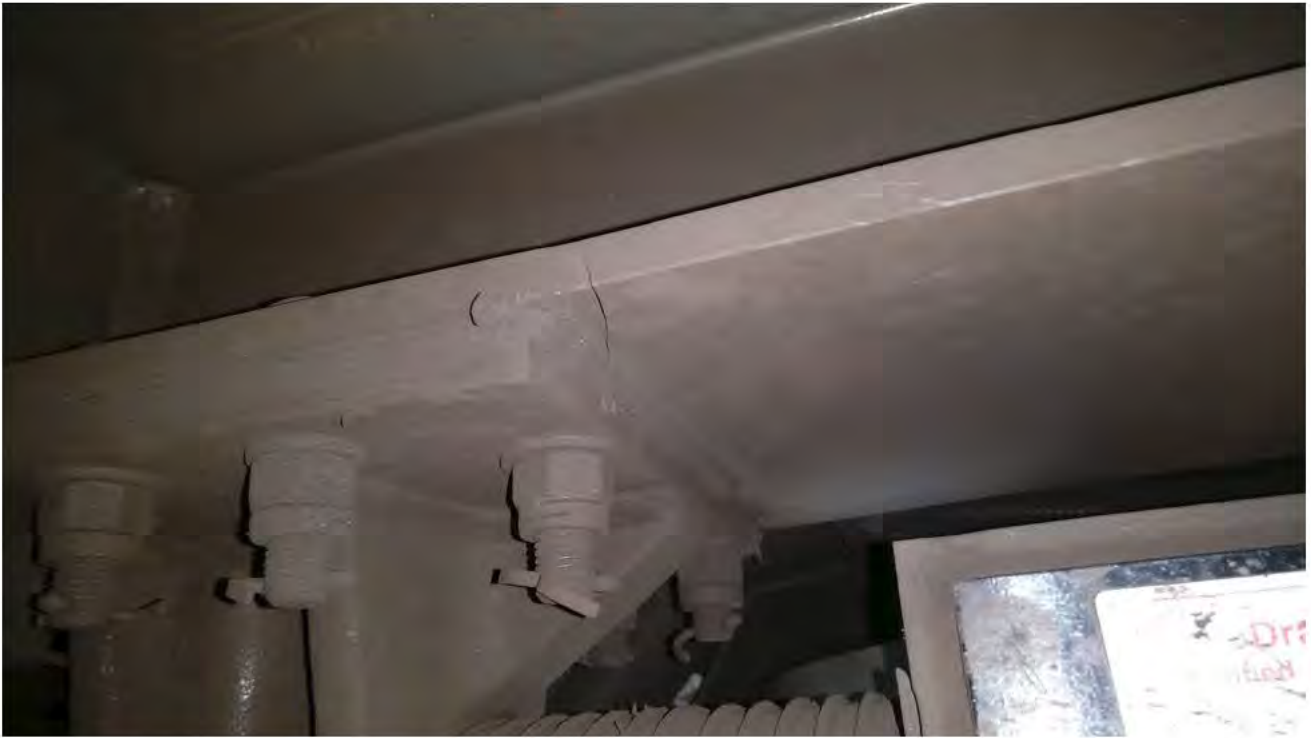
Figure 5: Image of car 96609 D End No. 1 side longitudinal beam fractures
