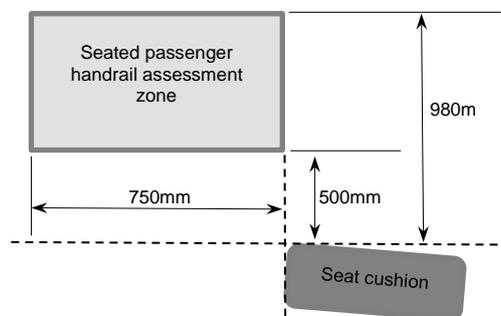
**Figure 46: Side view of seated passenger handrail assessment zone**
