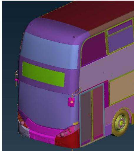
**Figure 26: Example CAD data required for bus vision standard assessment**
