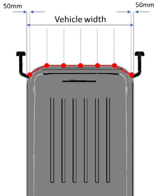
**Figure 3: Virtual profile for determining impact for VUT**
