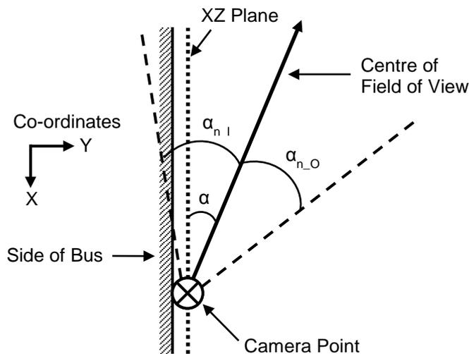
**Figure 19: Plan view of horizontal field of view range for camera point**
