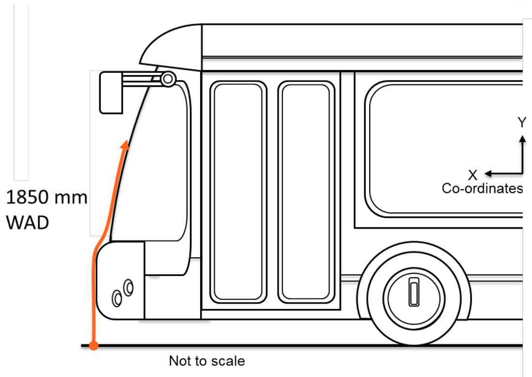
**Figure 64: Wrap around distance measurement**
