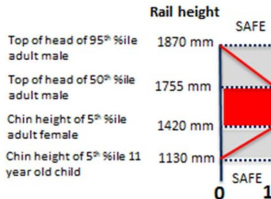
**Figure 54: Illustration of assessment for horizontal handrail based on its height above the bus floor.**
