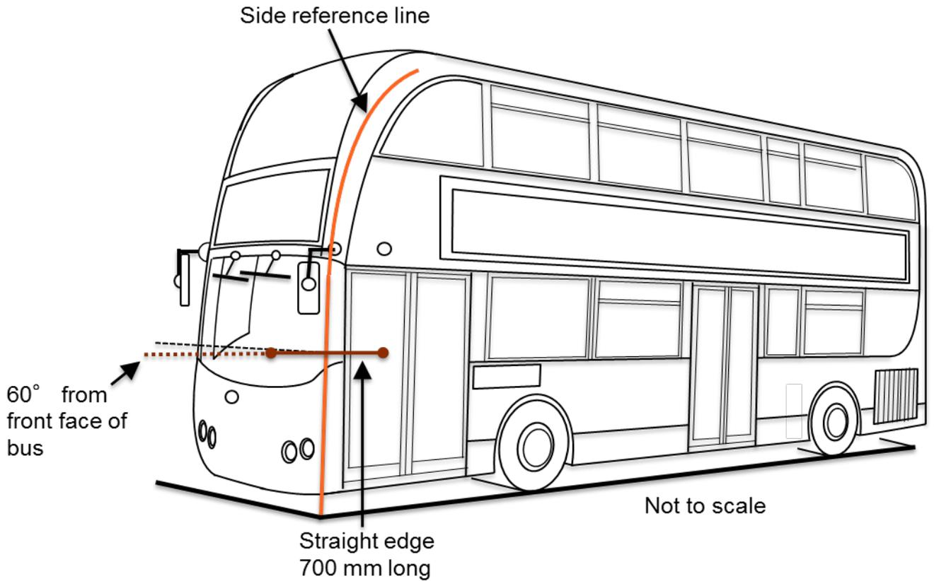
**Figure 2b: Side reference line – front/side view**
