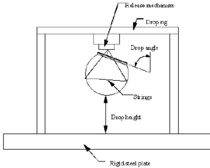
**Figure 68: Test set-up for dynamic headform impactor certification test**
