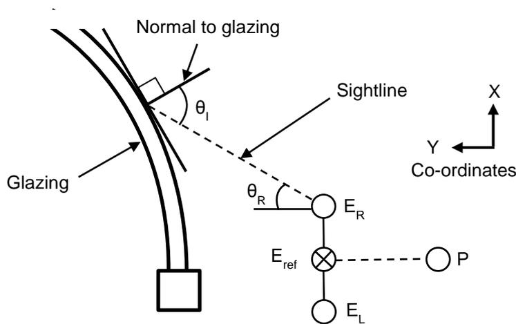
**Figure 28: Illustration of angle of incidence between the sightline and glazing**
