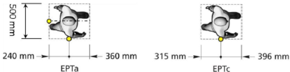
**Figure 4: Virtual box around EPT**
