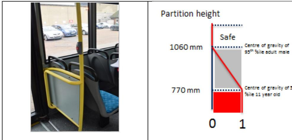
**Figure 55: Illustration of assessment of restraint (partitions) for standing passengers.**
