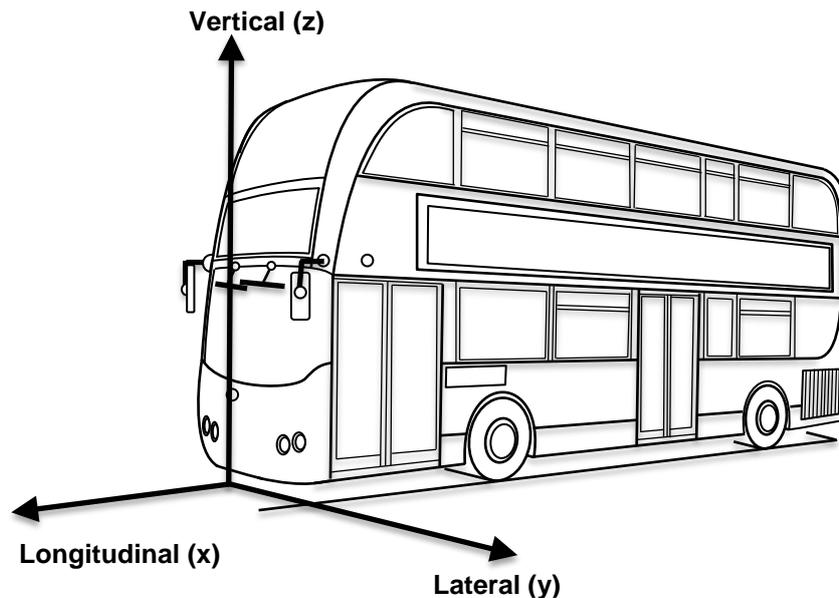
**Figure 25: Global coordinate system and notation**
