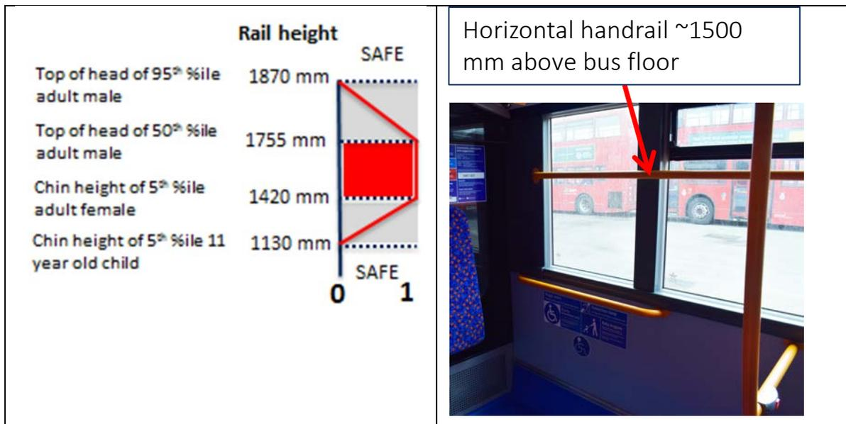
**Figure 60: Illustration of concept. Top rail in picture is about 1500 mm above the bus floor and in the red zone (and scores 1) whereas the bottom rail is about 1000 mm above the bus floor and in the safe zone (and scores 0). Grey zones, in which the score is scaled linearly from 1 to zero depending on the height of the rail above the bus floor, are positioned between the red and safe zones.**
