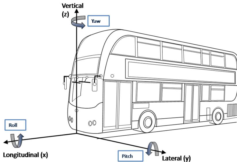
Figure 32: Local coordinate system and notation for test vehicle
