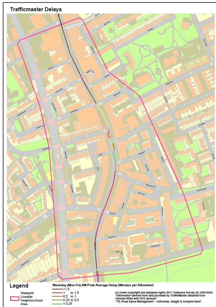
FIGURE 9. MAP OF AVERAGE DELAY. INFORMATION DERIVED FROM DATA PROVIDED BY TRAFFICMASTER OBTAINED FROM VEHICLES FITTED WITH GPS DEVICES
