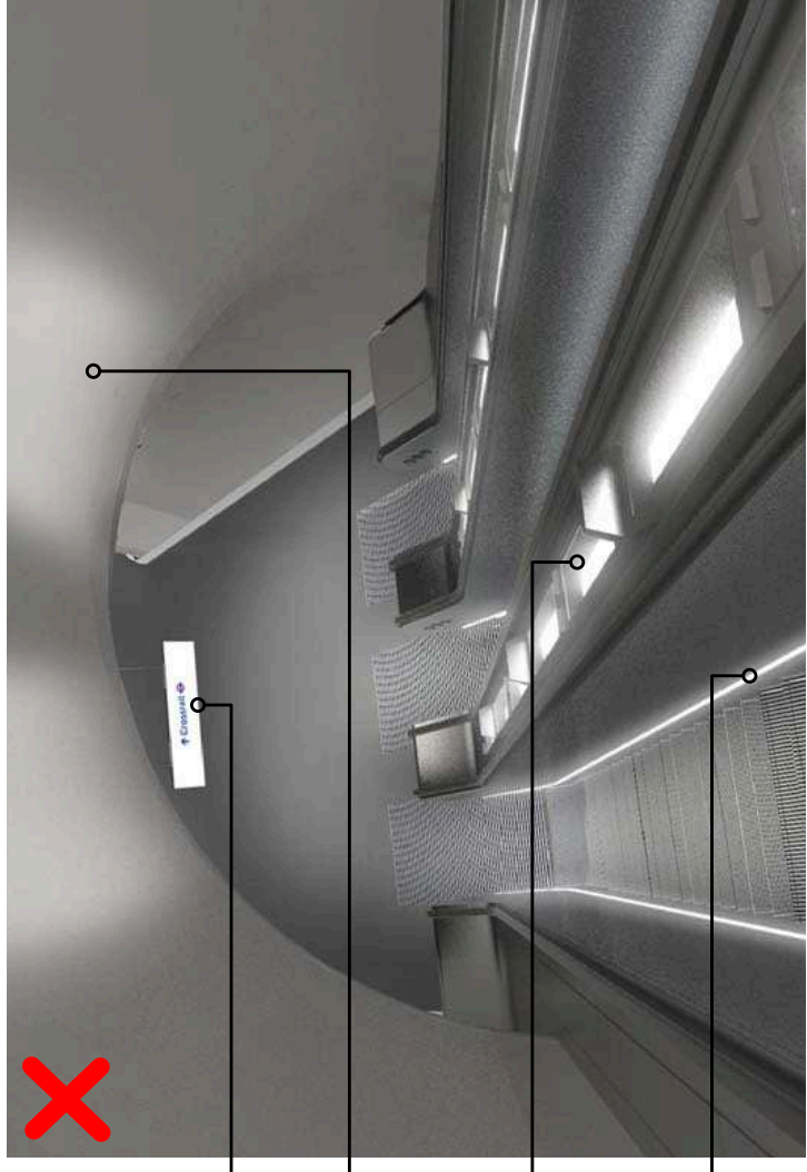
Deep-recessing of original SPL-502 deck uplight would compromise soft-edge illumination of vault
