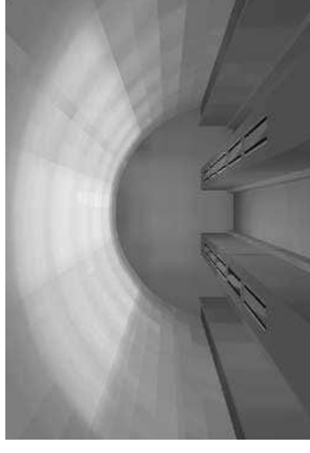
Dialux calc not accounting for diffusion - primary optic diffuser will blend beams & soften edges
