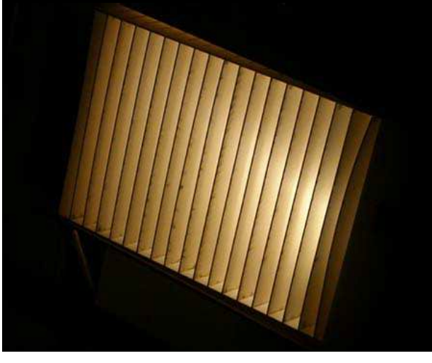
Lighter finish of secondary optic would reduce the perceived contrast between louvres and emitter and resultant patterning
