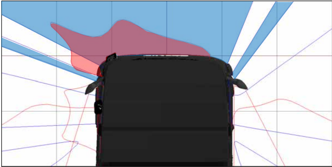
Figure 502. Image showing the areas of intersection of the projections of the driver's field of view through windows and mirrors. The blue areas show the projection of the windscreen and part of the side windows, the red areas the projection of the Class VI mirror, at a height above the ground that equals the stature of a 50th%ile UK male pedestrian
