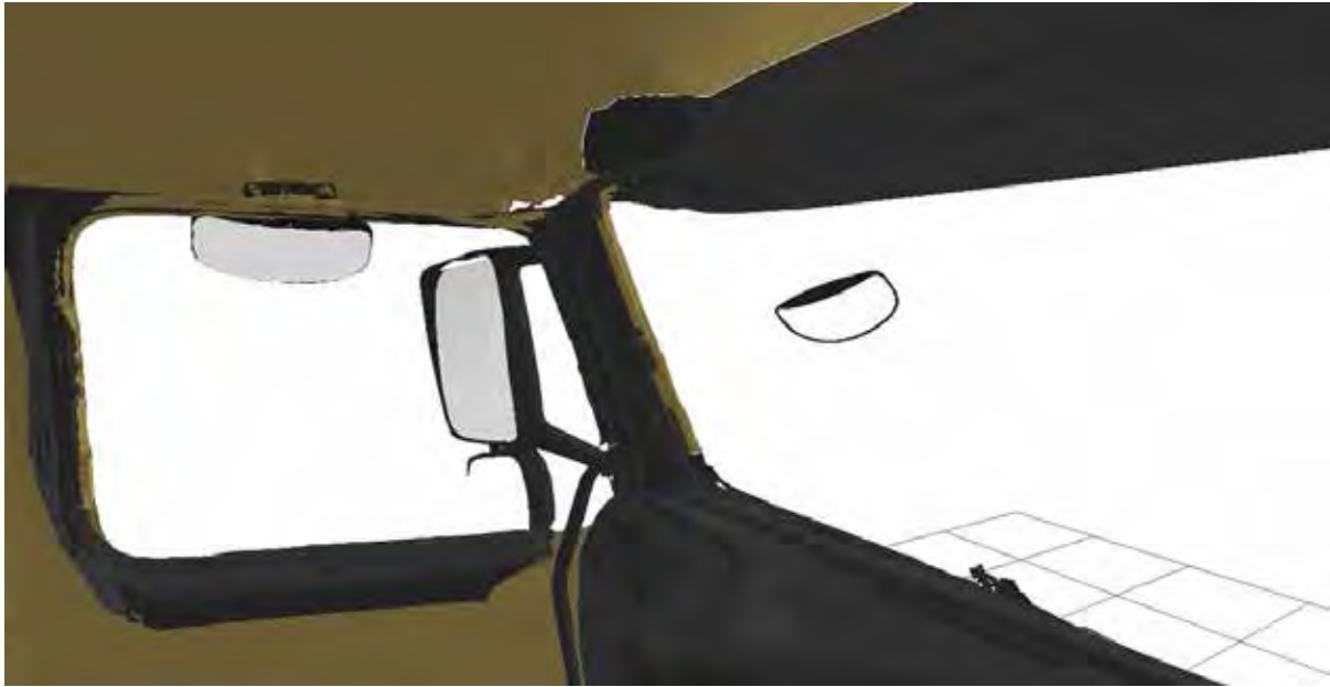
Figure 550. The view from the driver's eyes clearly shows the two cyclists are hidden from view.
