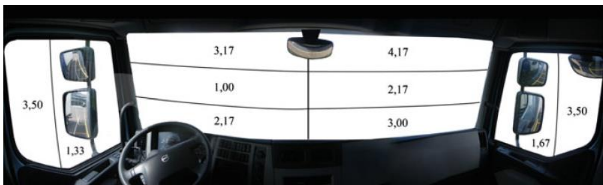
Figure 6-4: Importance of different window areas in the case of a distribution truck (1 means used most often, 5 means used most rarely). Source: (Terzis, 2016)
