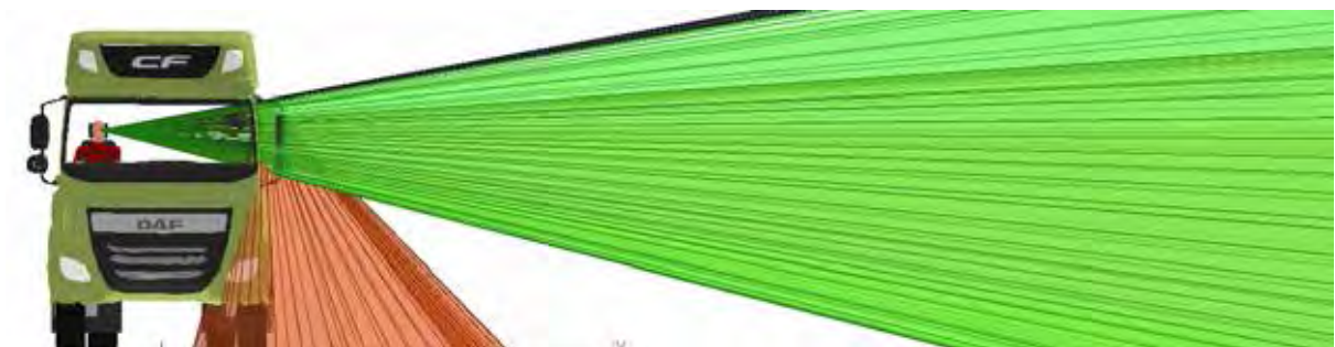
Figure 86. Combined projection of the near side windows and Class V mirror to the side of the DAF CF N3G
