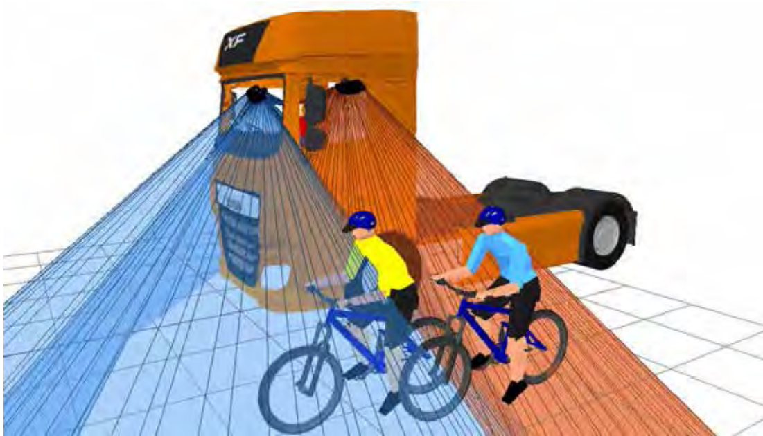
Figure 137. 3D view showing that both cyclists positioned to the nearside of the vehicle are visible in the projection of the Class V and / or Class VI mirrors
