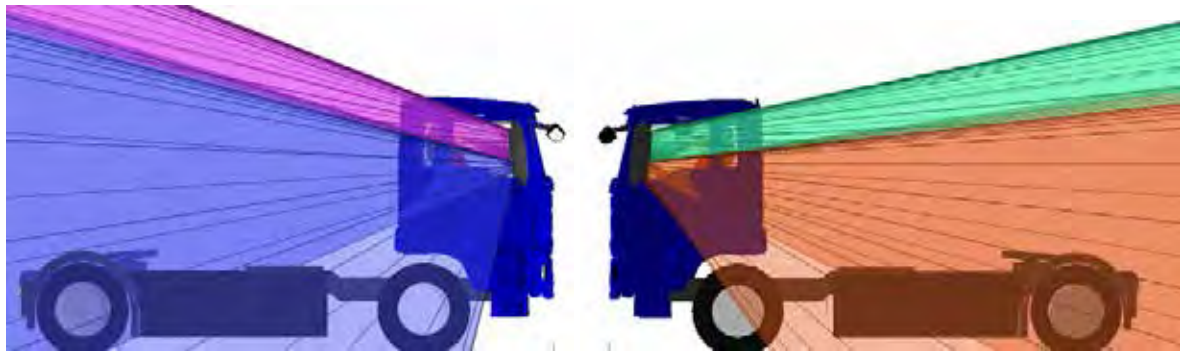
Figure 180. Side views of the combined Class II and Class IV mirror projections for the MAN TGS N3
