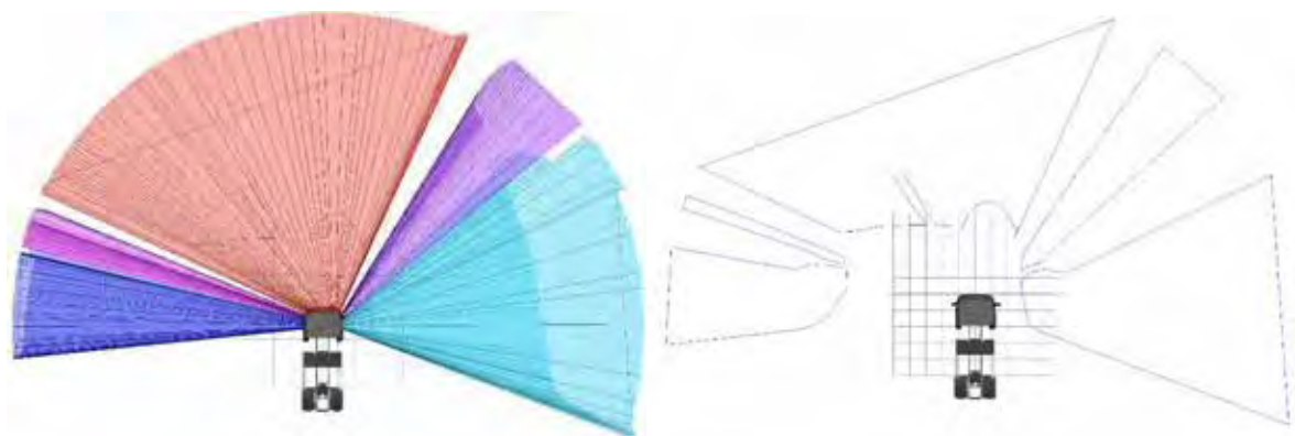
Figure 300. The projection of the windscreen and window apertures at the ground plane for the Mercedes Arocs N3G
