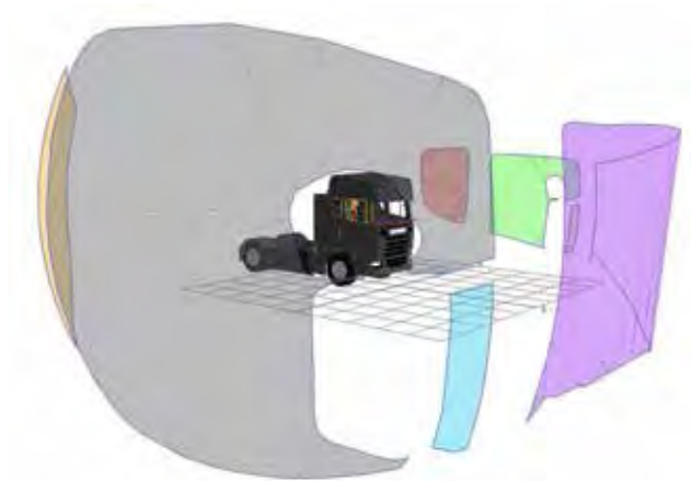
Figure 766. FOV area projection for the Scania R N3
