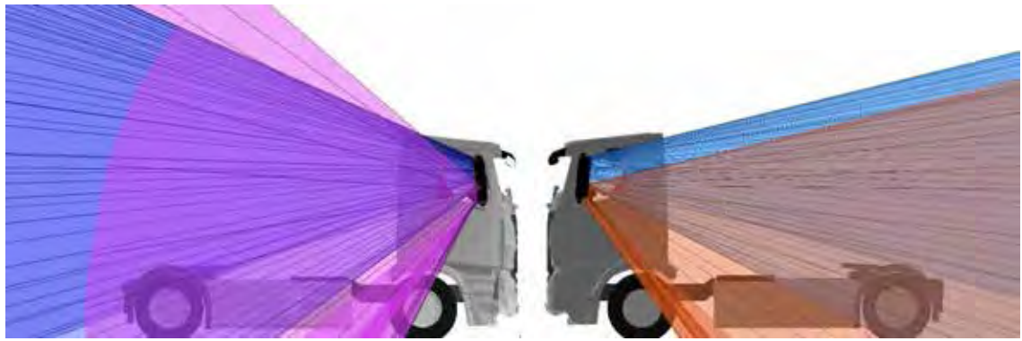
Figure 339. Side views of the combined Class II and Class IV mirror projections for the Mercedes Actros N3
