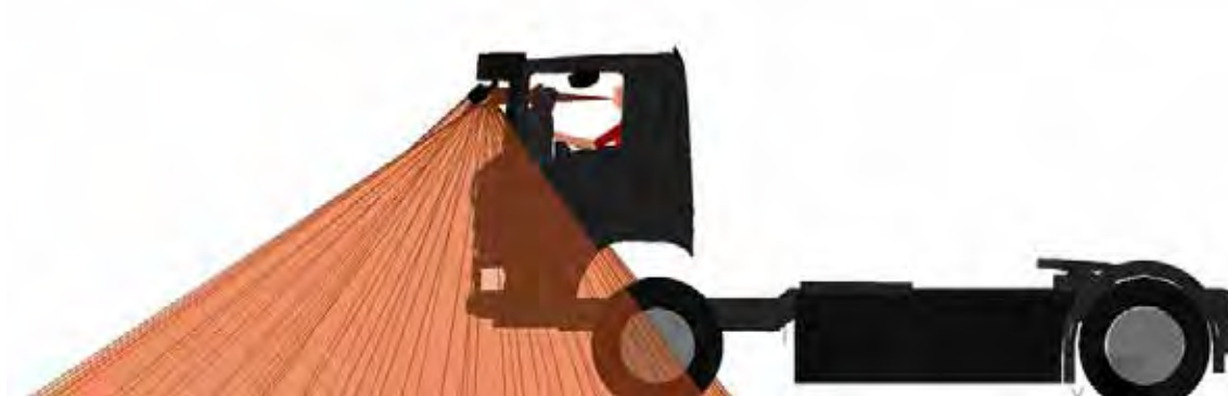
Figure 433. A side view of the Class VI mirror projection for the Scania P N3G
