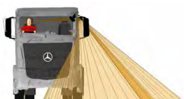
Figure 338. A front view of the Class V mirror projection for the Mercedes Actros N3
