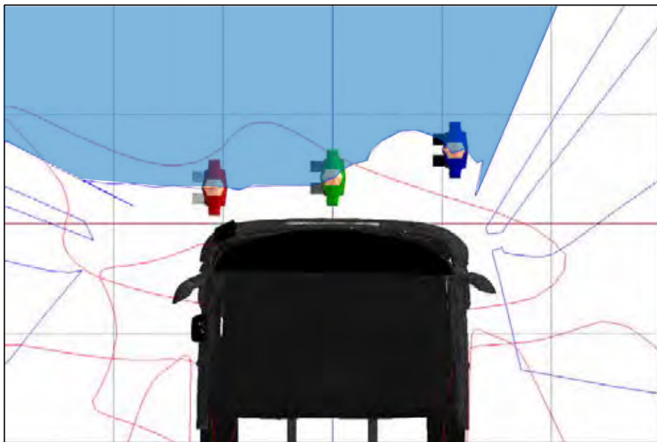
Figure 439. A plan view of the three human models that represent a pedestrian walking in front of a stationary vehicle and the projection of the windscreen at a height that equals the stature of a 50th%ile UK male pedestrian
