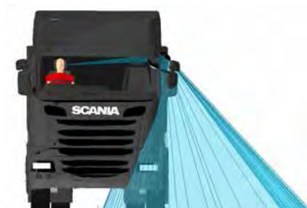
Figure 466. A front view of the Class V mirror projection for the Scania R N3
