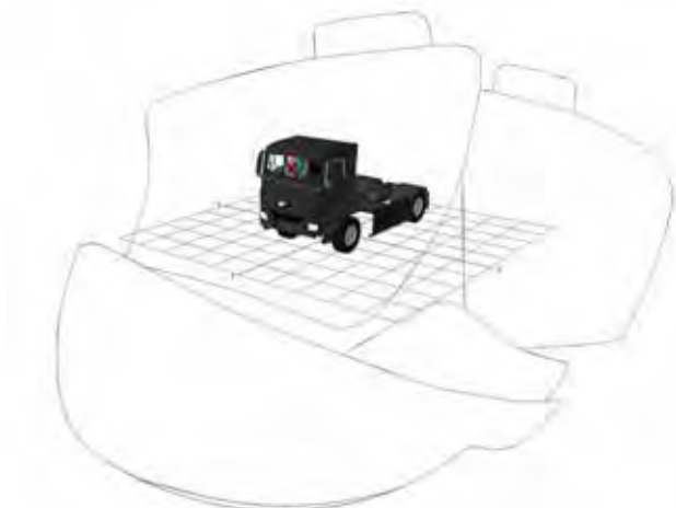
Figure 694. Combined indirect FOV area projection for the MAN TGS N3 / N3G
