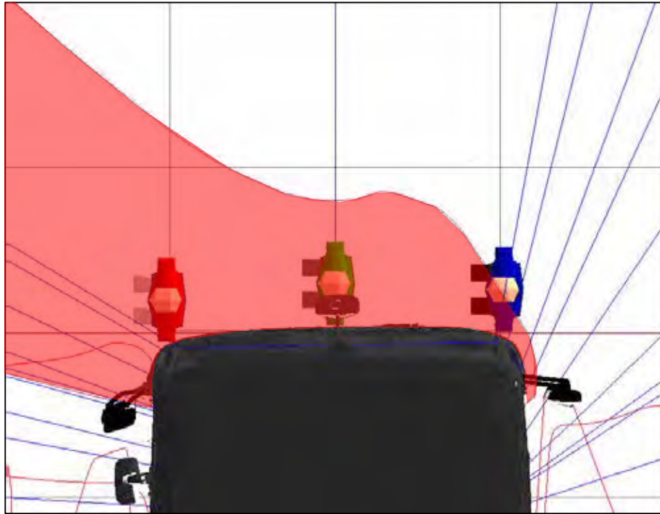
Figure 378. A plan view of the three human models that represent a pedestrian walking in front of a stationary vehicle and the projection of the Class VI mirror at a height that equals the stature of a 50th%ile UK male pedestrian
