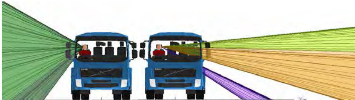
Figure 625. Frontal views of the off side and near side door window projections for the Volvo FE N3 LEC
