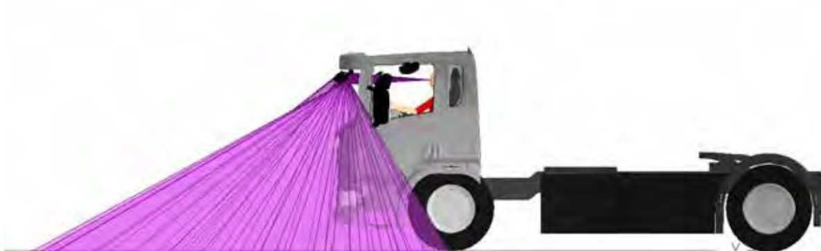
Figure 401. A side view of the Class VI mirror projection for the Scania P N3
