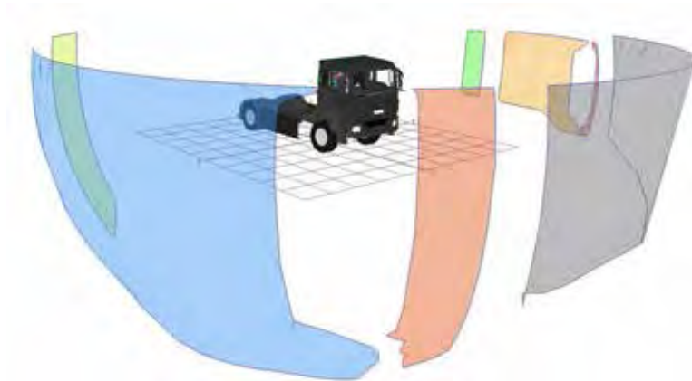
Figure 839. Clipped FOV area projection for the MAN TGS N3 / N3G
