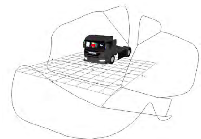
Figure 871. Combined indirect FOV area projection for the Scania N3 LEC
