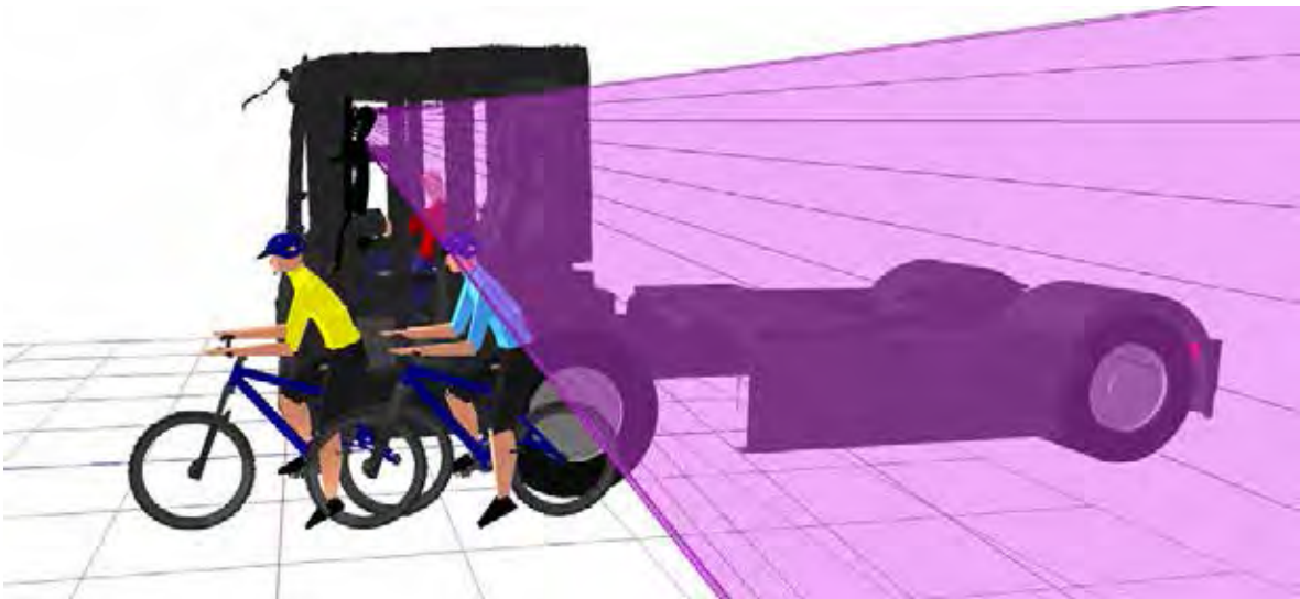
Figure 393. 3D view showing that the rear (blue) cyclist positioned to the nearside of the vehicle is visible in the projection of the Class IV mirror
