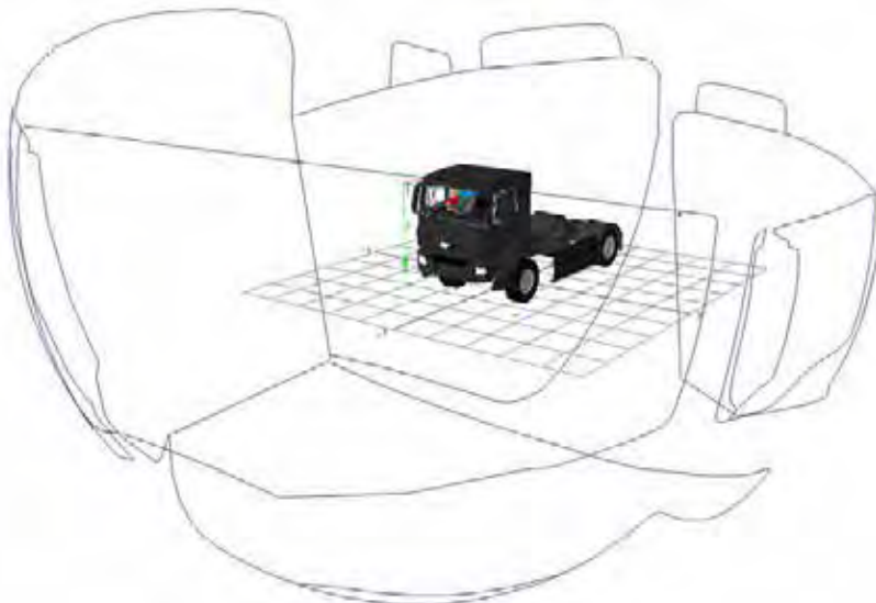
Figure 878. Combined direct and indirect FOV area projection for the MAN TGS N3 / N3G
