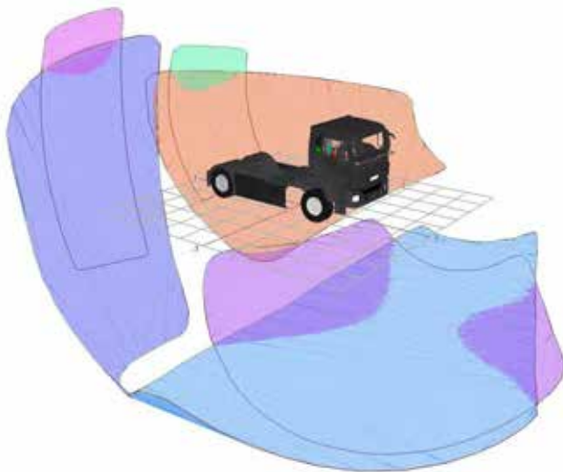
Figure 681. Indirect FOV area projection for the MAN TGS N3 / N3G
