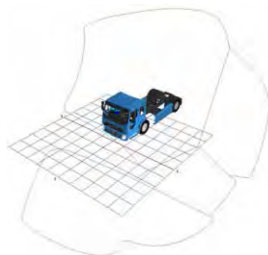
Figure 874. Combined indirect FOV area projection for the Volvo FE N3 LEC
