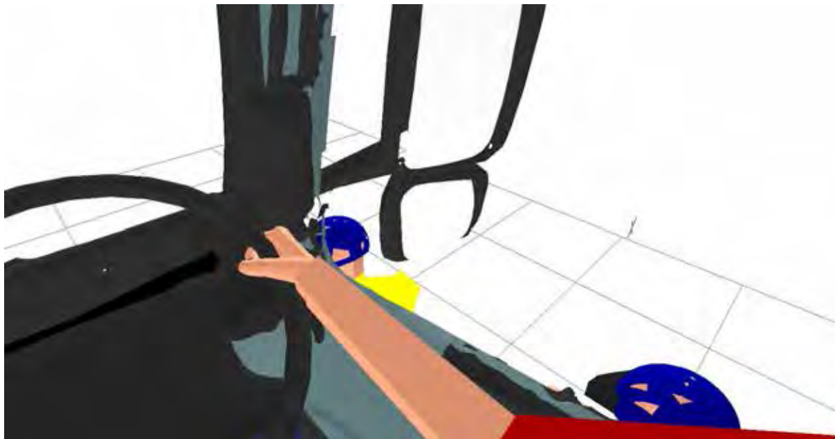
Figure 575. The view from the driver's eyes clearly shows the two cyclists are visible, even when positioned against the side of the vehicle.
