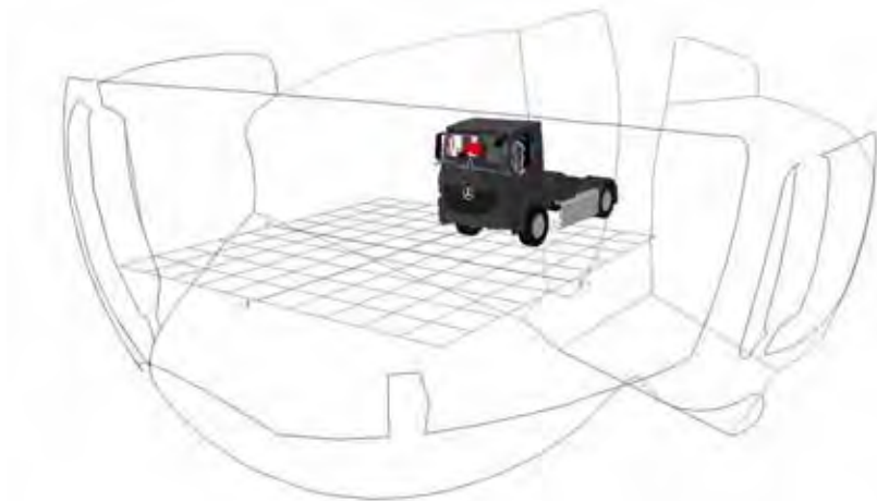
Figure 709. Combined direct and indirect FOV area projection for the Mercedes Antos N3 / Arocs N3G / Actros N3
