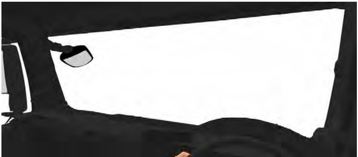
Figure 218. The view from the driver's eyes clearly shows the three pedestrians are hidden from view.
