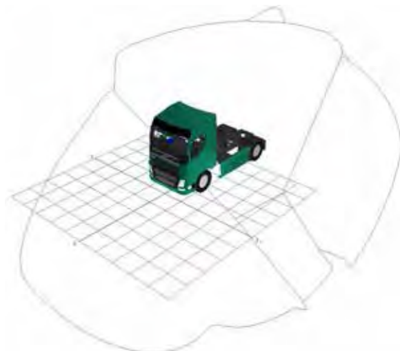
Figure 873. Combined indirect FOV area projection for the Volvo FH N3
