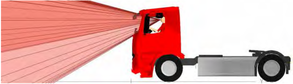
Figure 271. A side view of the windscreen aperture projection for the Mercedes Antos N3
