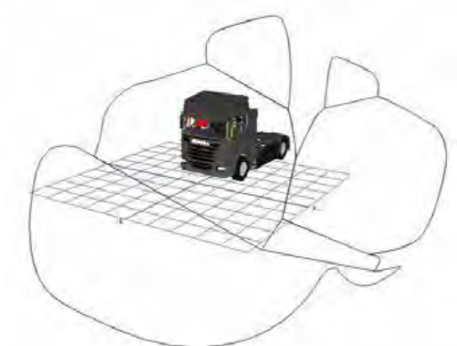
Figure 870. Combined indirect FOV area projection for the Scania R N3
