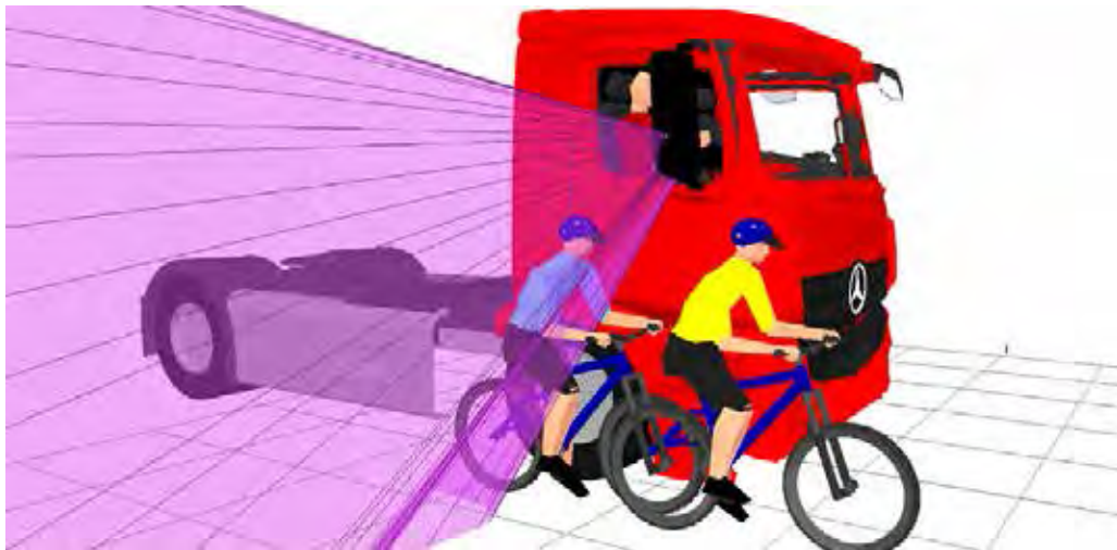
Figure 290. 3D view showing that the rear (blue) cyclist positioned to the offside of the vehicle is visible in the projection of the Class IV mirror
