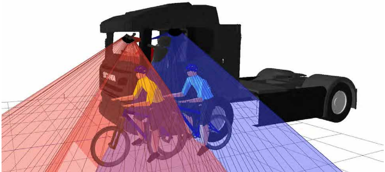
Figure 520. 3D view showing that the Front (yellow) cyclists positioned to the nearside of the vehicle is visible in the projection of the Class V and / or Class VI mirrors, and that the rear cyclist is visible in the Class V mirror
