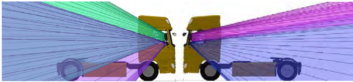
Figure 52. Side views of the combined Class II and Class IV mirror projections for the DAF CF N3
