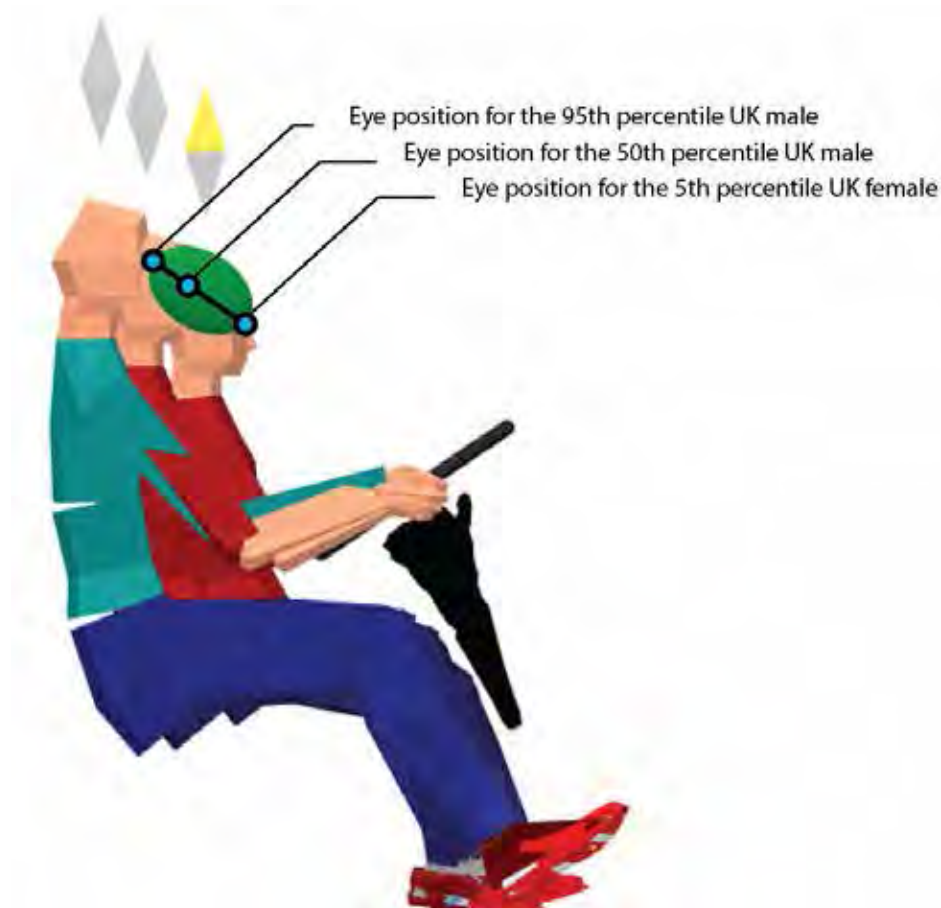
Figure 8. An example of the postures that were defined by the location of the Eyellipse and the available adjustability of the seat and steering wheel
