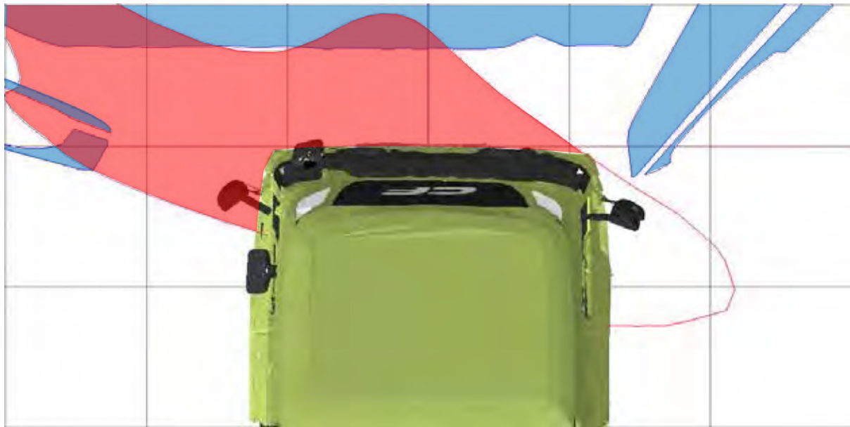
Figure 87. Image showing the areas of intersection of the projections of the driver's field of view through windows and mirrors. The blue areas show the projection of the windscreen and part of the side windows, the red areas the projection of the Class VI mirror, at a height above the ground that equals the stature of a 50th%ile UK male pedestrian
