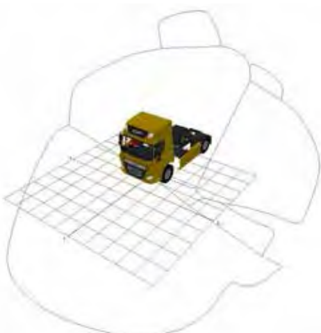
Figure 797. Combined indirect FOV area projection for the DAF CF N3 / N3G
