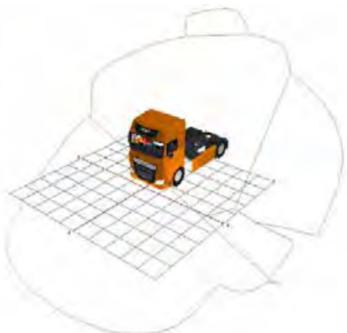
Figure 692. Combined indirect FOV area projection for the DAF XF N3
