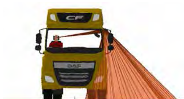
Figure 51. A front view of the Class V mirror projection for the DAF CF N3
