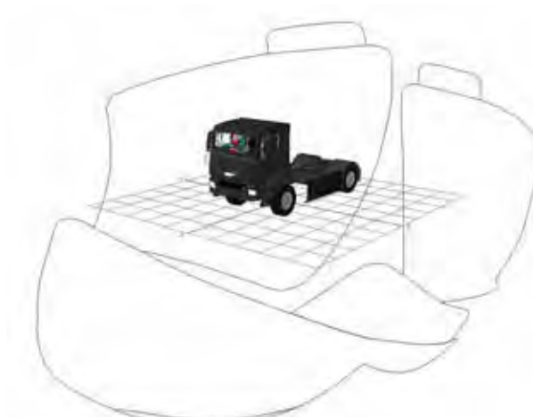
Figure 865. Combined indirect FOV area projection for the MAN TGS N3 / N3G
