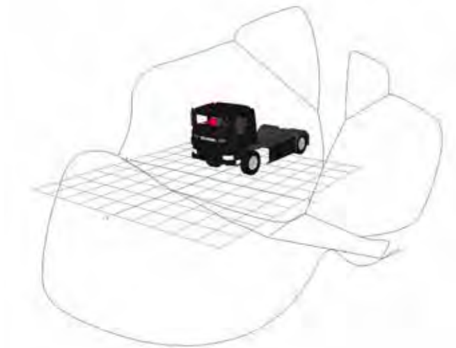
Figure 804. Combined indirect FOV area projection for the Scania P N3 / N3G
