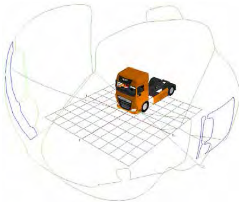
Figure 811. Combined direct and indirect FOV area projection for the DAF XF N3
