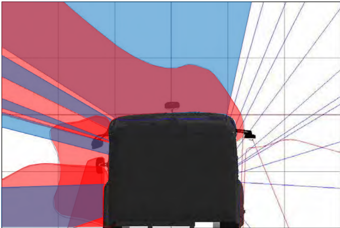
Figure 387. Image showing the areas of intersection of the projections of the driver's field of view through windows and mirrors. The blue areas show the projection of the windscreen and the nearside windows, the red areas show the projection of the Class II, Class IV, Class V and Class VI mirrors, at a height above the ground that equals the height of a 50th%ile UK male cyclist
