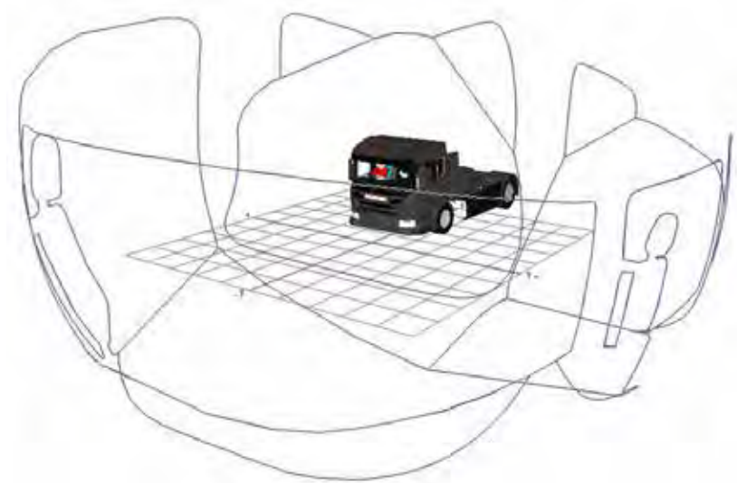
Figure 713. Combined direct and indirect FOV area projection for the Scania N3 LEC
