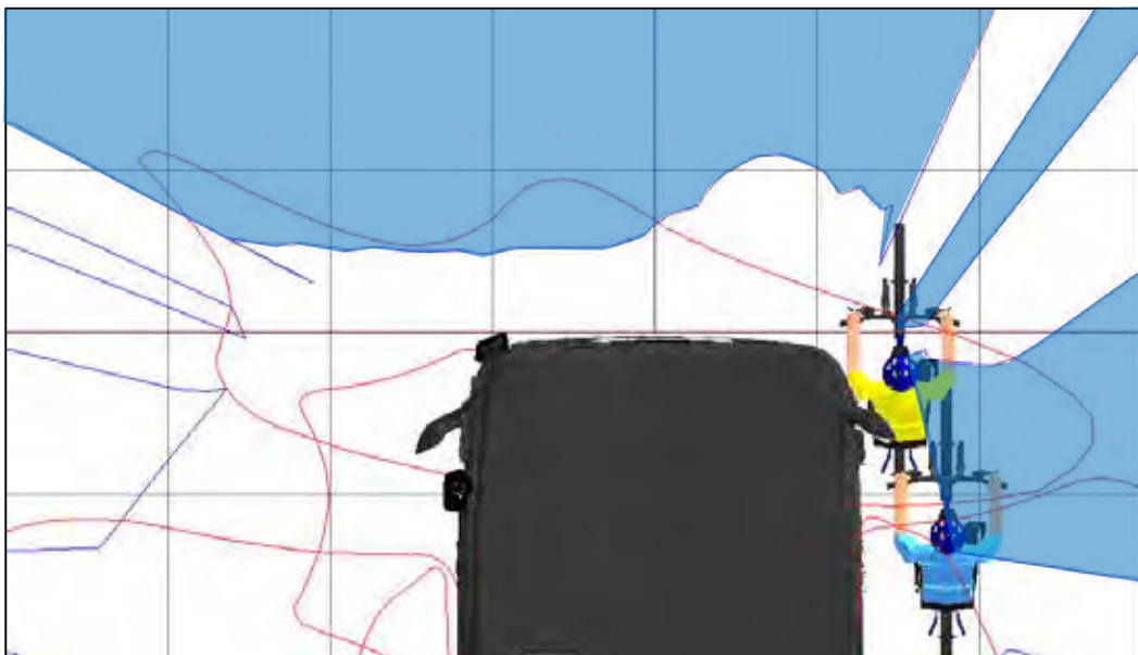
Figure 477. A plan view of the two human models that represent a cyclist moving past on the outside of the vehicle and the projection of the windscreen and offside windows at a height that equals the stature of a 50th%ile UK male cyclist
