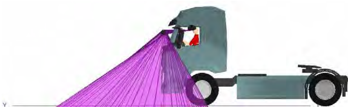
Figure 561. A side view of the Class VI mirror projection for the Volvo FMX N3G
