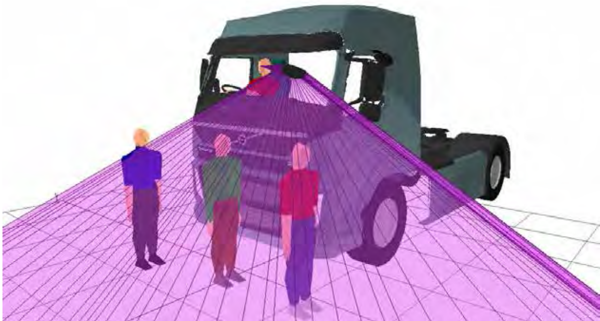
Figure 571. 3D view showing that all three pedestrians positioned to the front of the vehicle are visible in the projection of the Class VI mirror
