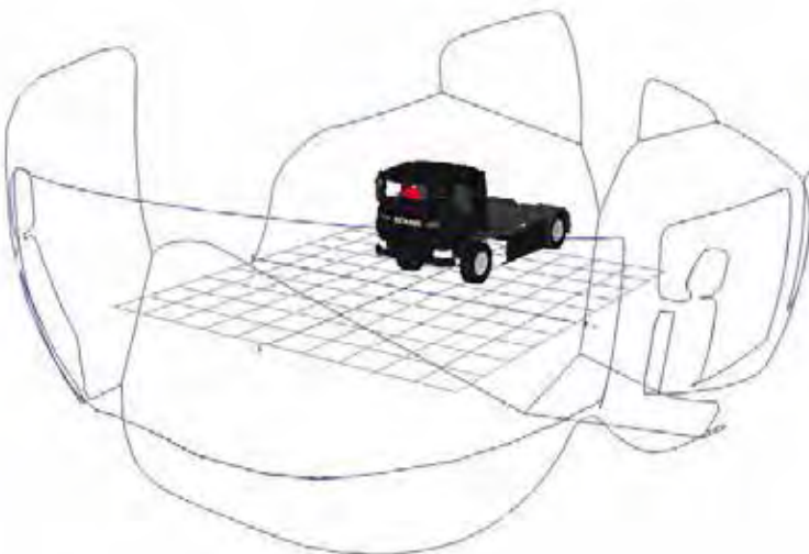
Figure 882. Combined direct and indirect FOV area projection for the Scania P N3 / N3G
