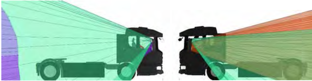
Figure 499. Side views of the combined Class II and Class IV mirror projections for the Scania N3 LEC
