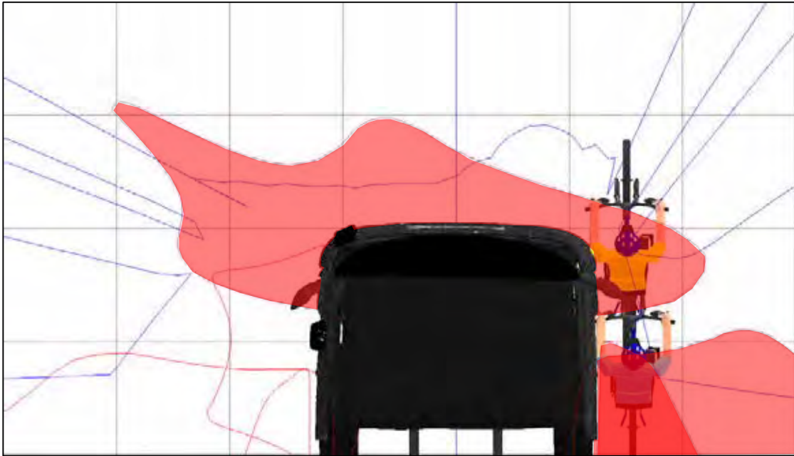
Figure 448. A plan view of the two human models that represent a cyclist moving past on the outside of the vehicle and the projection of the Class IV and Class VI mirrors at a height that equals the stature of a 50th%ile UK male cyclist
