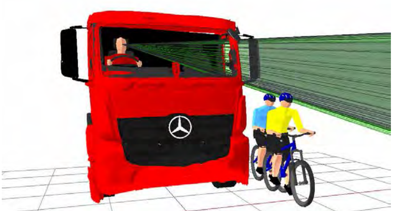
Figure 293. 3D view showing that the two human models can be positioned 359mm (yellow) and 300mm (blue) to the side of the vehicle without being seen through direct vision by the driver in the standardised driving posture
