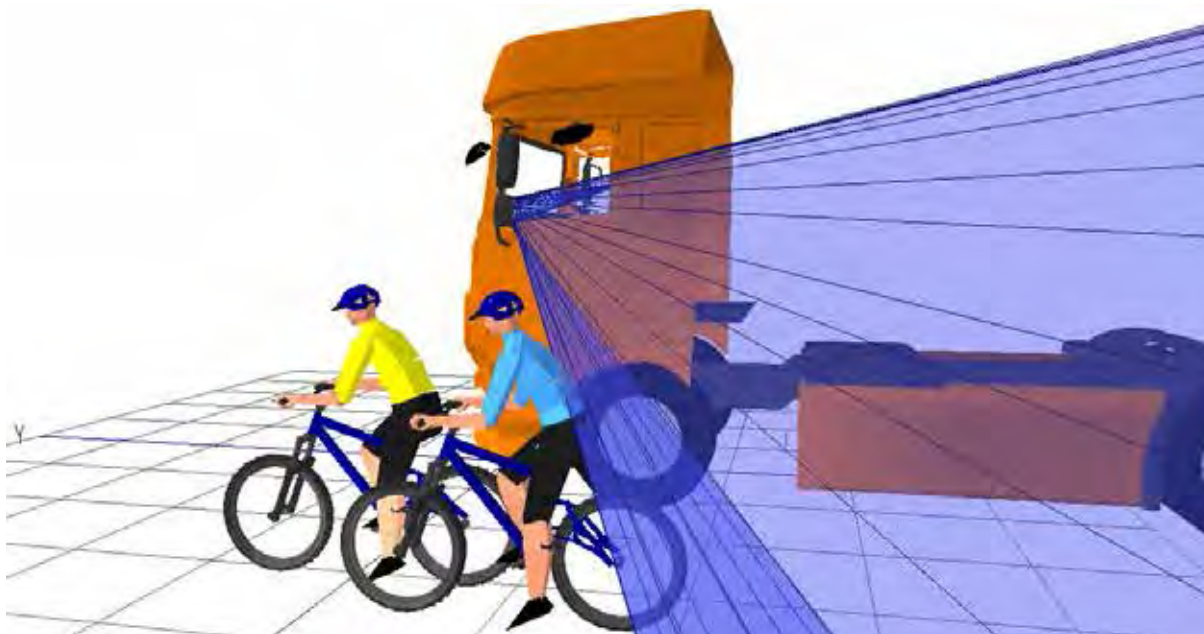
Figure 138. 3D view showing that the rear (blue) cyclist positioned to the nearside of the vehicle is barely visible in the projection of the Class IV mirror
