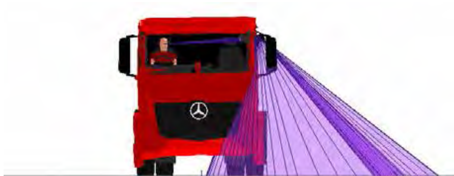
Figure 274. A front view of the Class V mirror projection for the Mercedes Antos N3
