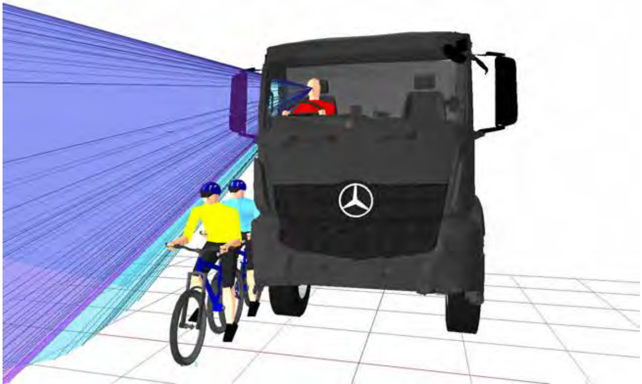
Figure 318. 3D view showing that both cyclists can be hidden from direct vision to the offside of the Mercedes Arocs N3G
