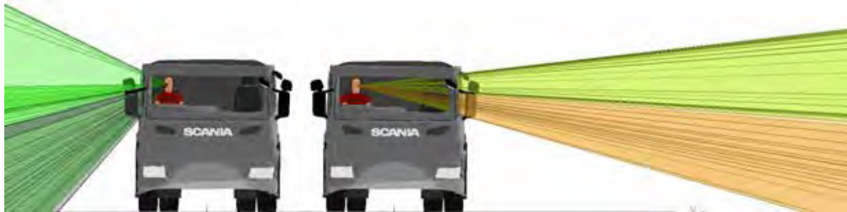
Figure 400. Frontal views of the off side and near side door window projections for the Scania P N3
