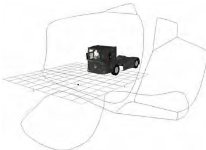
Figure 868. Combined indirect FOV area projection for the Mercedes Econic N3 LEC
