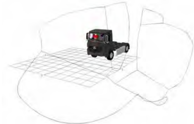
Figure 696. Combined indirect FOV area projection for the Mercedes Antos N3 / Arocs N3G / Actros N3
