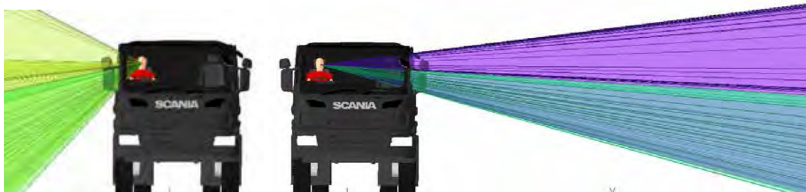
Figure 432. Frontal views of the off side and near side door window projections for the Scania P N3G
