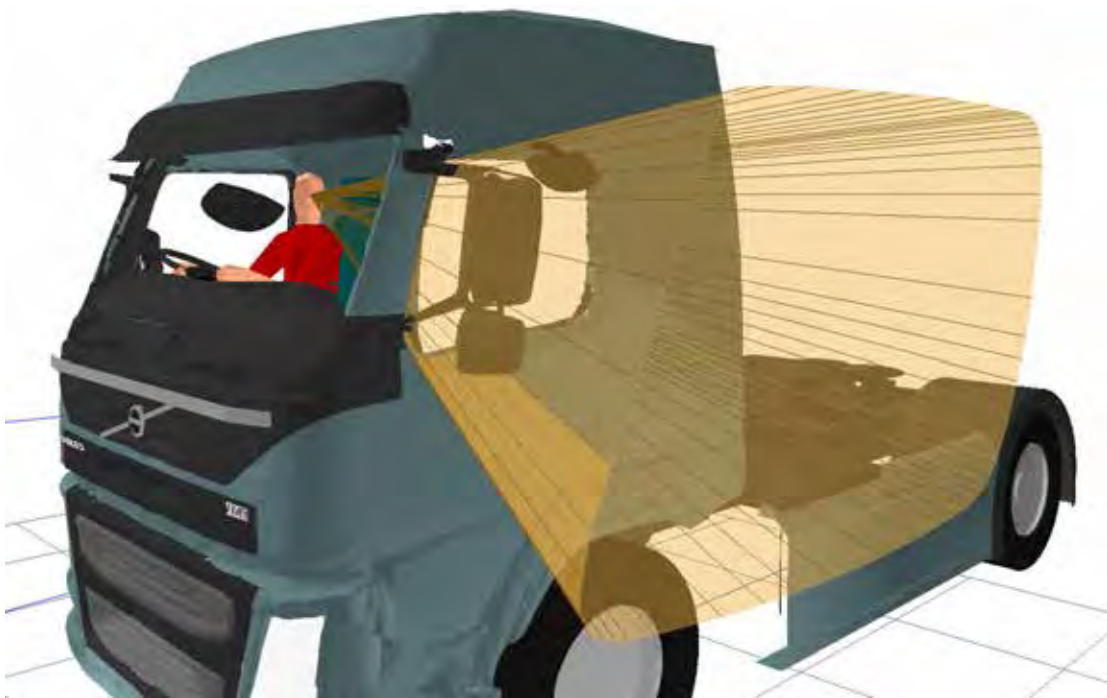
Figure 16. Volumetric projection of the nearside window.
