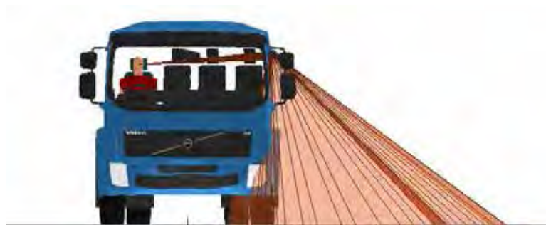
Figure 627. A front view of the Class V mirror projection for the Volvo FE N3 LEC
