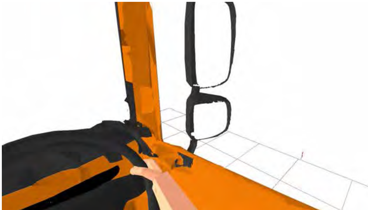
Figure 128. The view from the driver's eyes shows the two cyclists are hidden from view.
