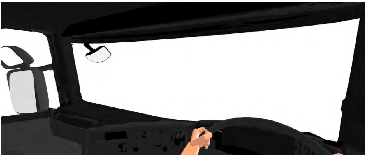
Figure 441. The view from the driver's eyes clearly shows the three pedestrians are hidden from view.
