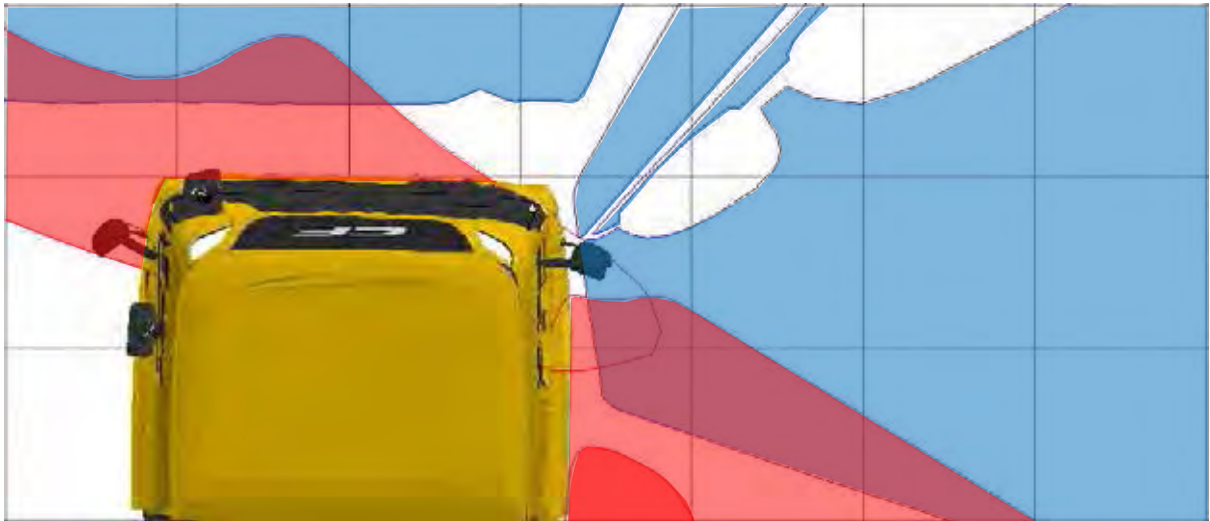
Figure 61. Image showing the areas of intersection of the projections of the driver's field of view through windows and mirrors. The blue areas show the projection of the windscreen and the offside windows, the red areas show the projection of the Class II, Class IV and Class VI mirrors, at a height above the ground that equals the height of a 50th%ile UK male cyclist
