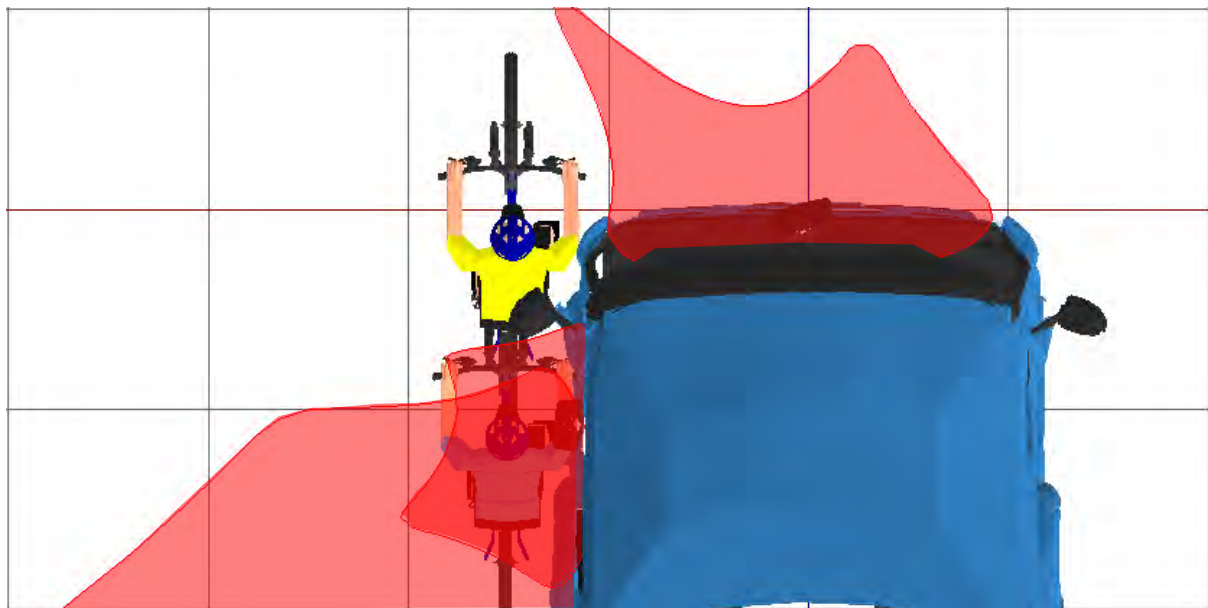
Figure 648. A plan view of the two human models that represent a cyclist moving up the inside of the vehicle and the projection of the Class IV, Class V and Class VI mirrors at a height that equals the stature of a 50th%ile UK male cyclist
