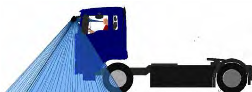
Figure 178. A side view of the Class VI mirror projection for the MAN TGS N3
