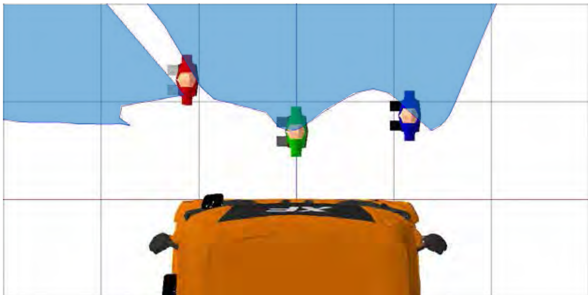
Figure 120. A plan view of the three human models that represent a pedestrian walking in front of a stationary vehicle and the projection of the windscreen at a height that equals the stature of a 50th%ile UK male pedestrian
