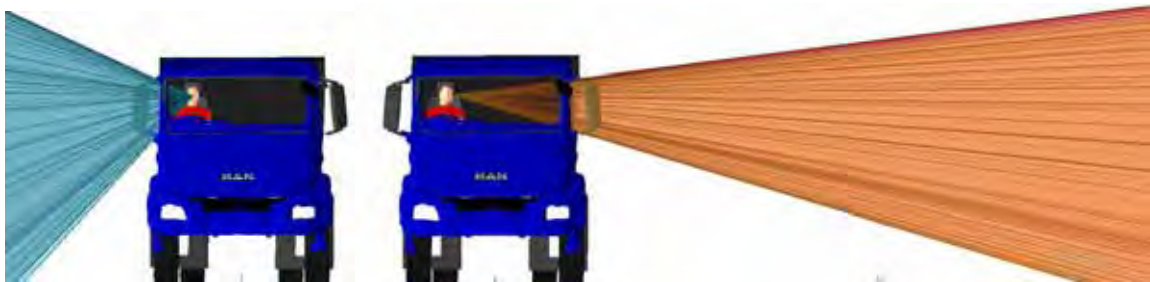
Figure 177. Frontal views of the off side and near side door window projections for the MAN TGS N3
