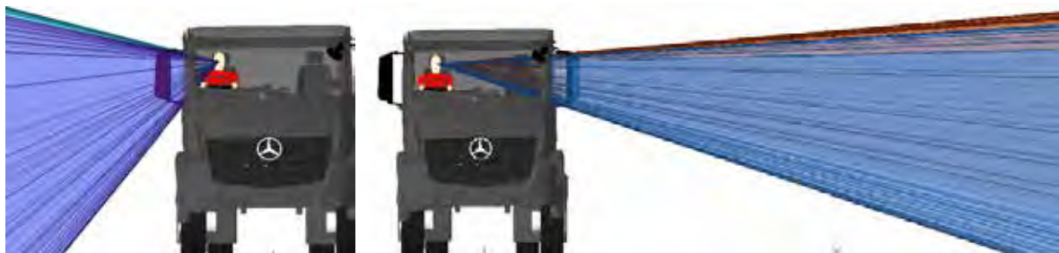
Figure 304. Frontal views of the off side and near side door window projections for the Mercedes Arocs N3G
