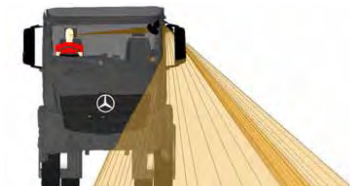
Figure 306. A front view of the Class V mirror projection for the Mercedes Arocs N3G
