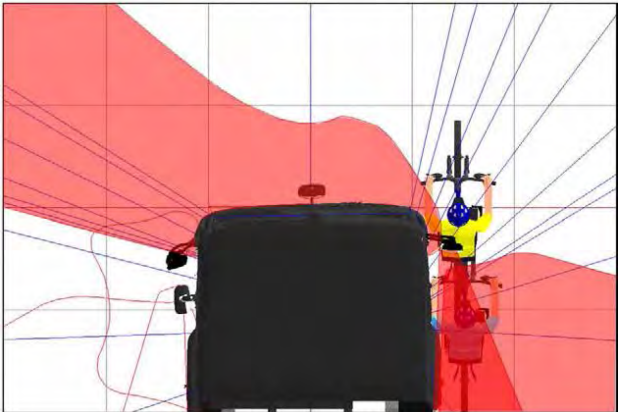
Figure 384. A plan view of the two human models that represent a cyclist moving past on the outside of the vehicle and the projection of the Class IV and Class VI mirrors at a height that equals the stature of a 50th%ile UK male cyclist
