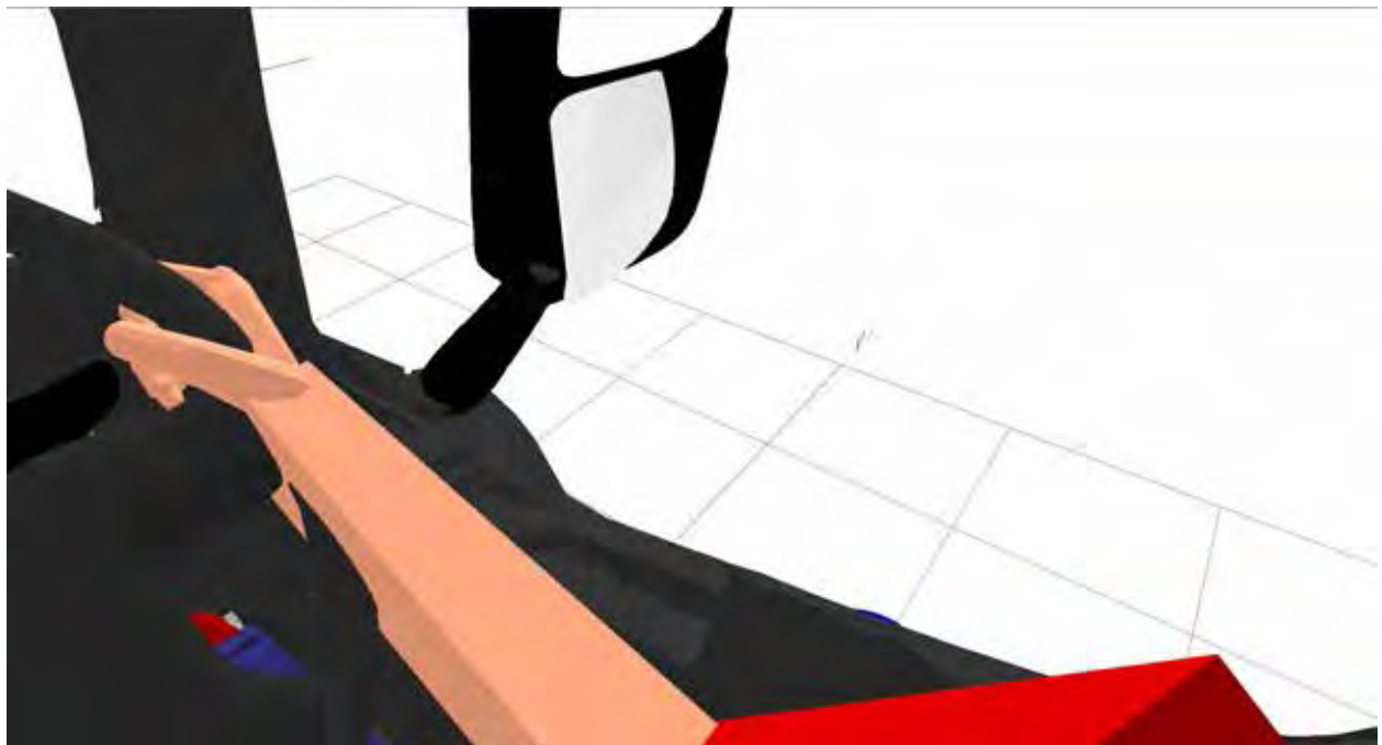
Figure 319. The view from the driver's eyes clearly shows the two cyclists are not visible
