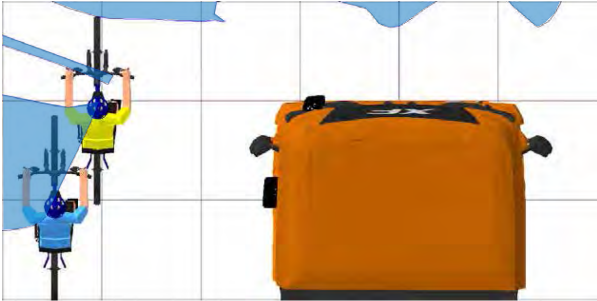
Figure 133. A plan view of the two human models that represent a cyclist moving up the inside of the vehicle and the projection of the windscreen and nearside windows at a height that equals the stature of a 50th%ile UK male cyclist
