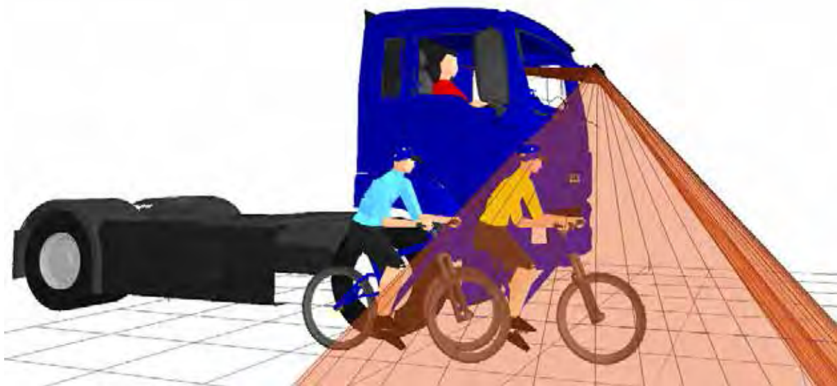
Figure 194. 3D view showing that the front (yellow) cyclist positioned to the offside of the vehicle is visible in the projection of the Class VI
