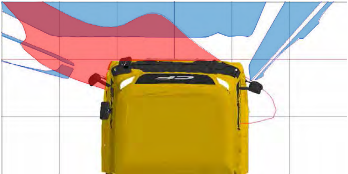
Figure 55. Image showing the areas of intersection of the projections of the driver's field of view through windows and mirrors. The blue areas show the projection of the windscreen and part of the side windows, the red areas the projection of the Class VI mirror, at a height above the ground that equals the stature of a 50th%ile UK male pedestrian
