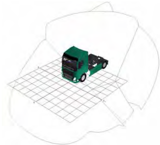
Figure 702. Combined indirect FOV area projection for the Volvo FH N3
