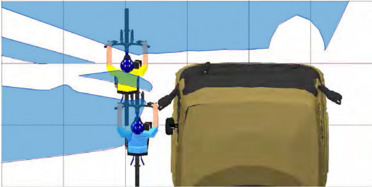
Figure 548. A plan view of the two human models that represent a cyclist moving up the inside of the vehicle and the projection of the windscreen and nearside windows at a height that equals the stature of a 50th%ile UK male cyclist
