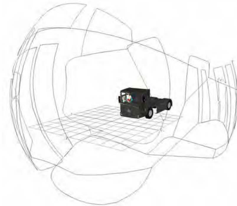
Figure 816. Combined direct and indirect FOV area projection for the Mercedes Econic N3 LEC
