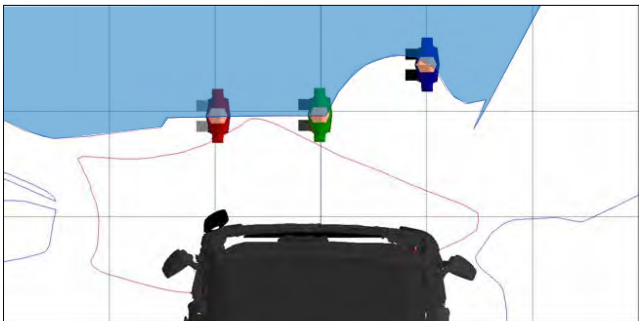
Figure 216. A plan view of the three human models that represent a pedestrian walking in front of a stationary vehicle and the projection of the windscreen at a height that equals the stature of a 50th%ile UK male pedestrian
