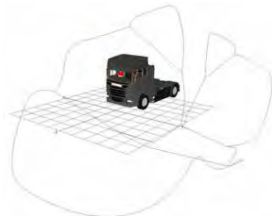
Figure 805. Combined indirect FOV area projection for the Scania R N3
