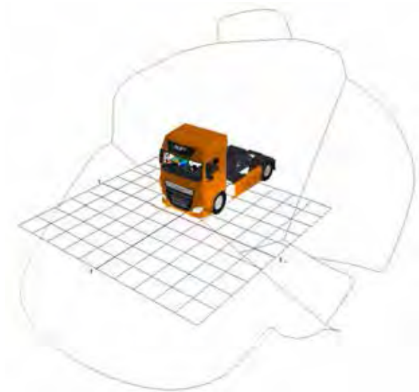
Figure 863. Combined indirect FOV area projection for the DAF XF N3
