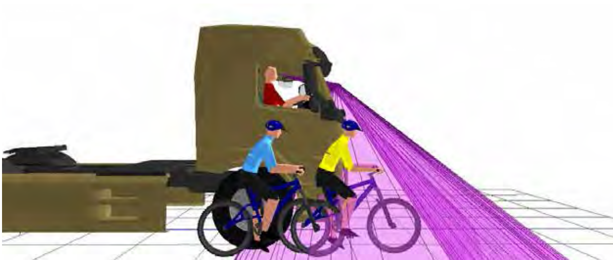
Figure 545. 3D view showing that the front (yellow) cyclist positioned to the offside of the vehicle is visible in the projection of the Class VI
