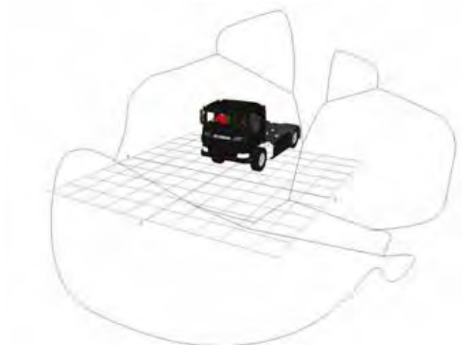
Figure 698. Combined indirect FOV area projection for the Scania P N3 / N3G
