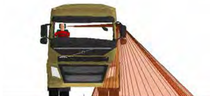
Figure 530. A front view of the Class V mirror projection for the Volvo FM N3
