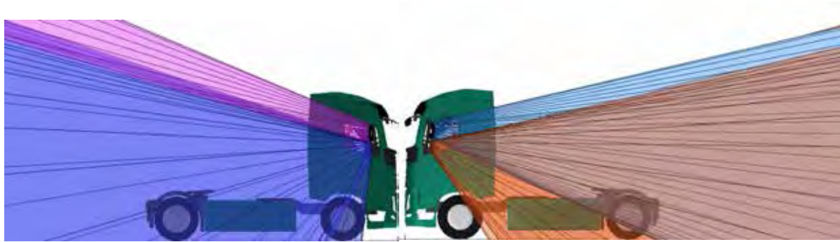
Figure 595. Side views of the combined Class II and Class IV mirror projections for the Volvo FH N3
