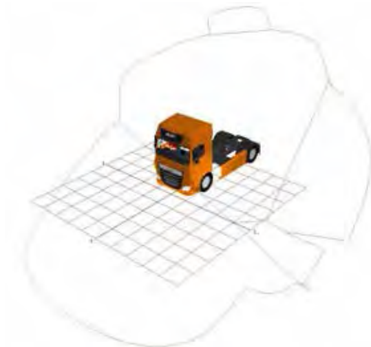
Figure 798. Combined indirect FOV area projection for the DAF XF N3
