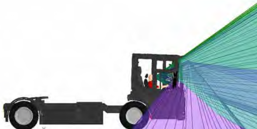
Figure 372. Combined projection of the windscreen and Class VI mirror to the front of the Mercedes Econic LEC
