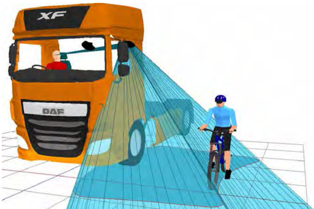
Figure 19. Image showing how objects within the 2D projection area, may not be visible to the driver
