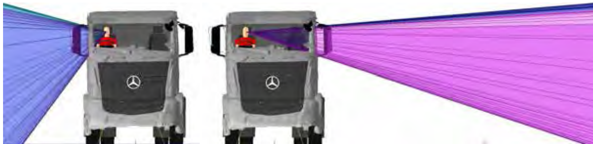
Figure 336. Frontal views of the off side and near side door window projections for the Mercedes Actros N3
