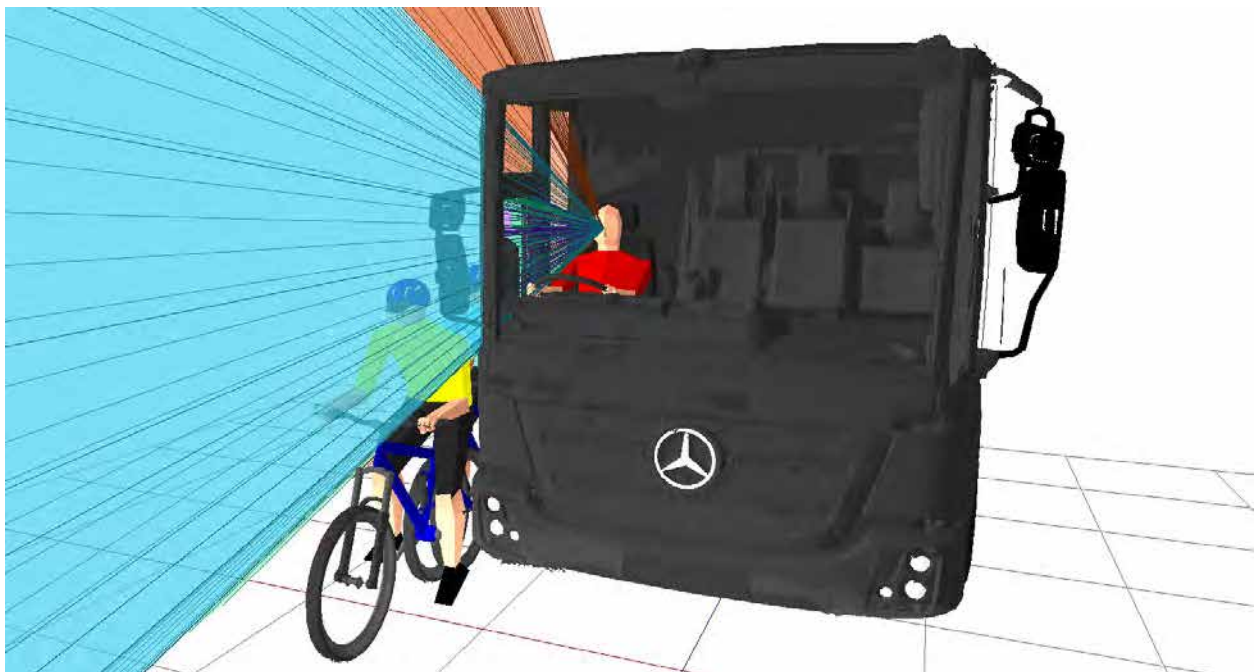
Figure 382. 3D view showing that both cyclists cannot be hidden from direct vision to the offside of the Dennis Eagle Elite 6
