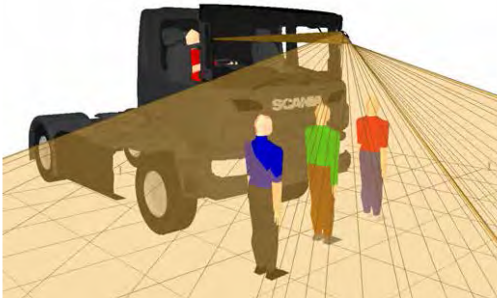
Figure 443. 3D view showing that all three pedestrians positioned to the front of the vehicle are visible in the projection of the Class VI mirror
