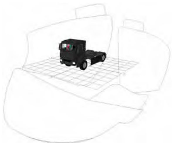
Figure 800. Combined indirect FOV area projection for the MAN TGS N3 / N3G
