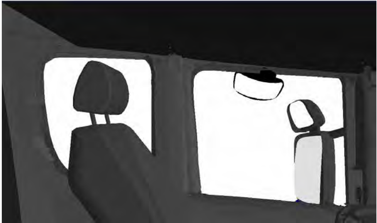
Figure 486. The view from the driver's eyes clearly shows the two cyclists are hidden from view.
