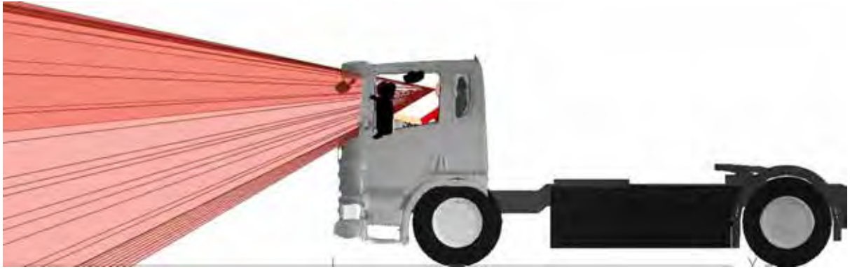
Figure 399. A side view of the windscreen aperture projection for the Scania P N3
