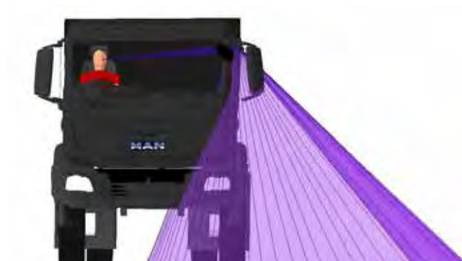
Figure 211. A front view of the Class V mirror projection for the MAN TGS N3G
