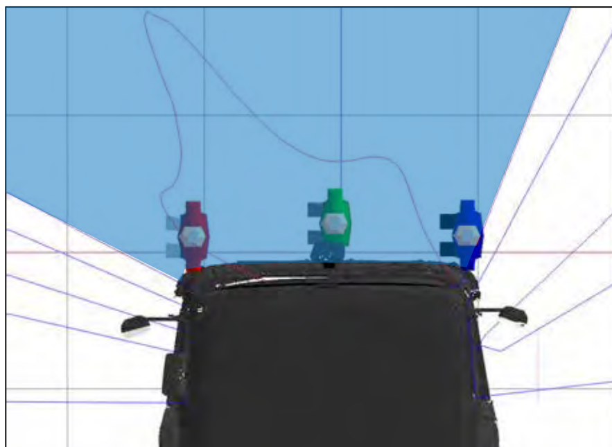
Figure 152. A plan view of the three human models that represent a pedestrian walking in front of a stationary vehicle and the projection of the windscreen at a height that equals the stature of a 50th%ile UK male pedestrian
