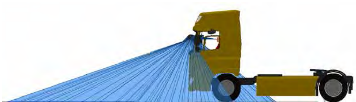
Figure 50. A side view of the Class VI mirror projection for the DAF CF N3
