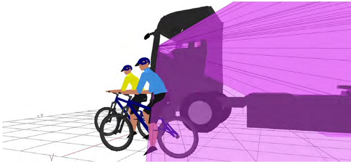
Figure 265. 3D view showing that the rear (blue) cyclist positioned to the nearside of the vehicle is visible in the projection of the Class IV mirror
