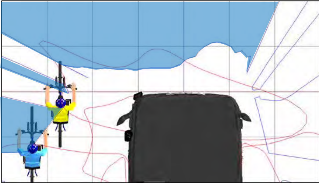
Figure 484. A plan view of the two human models that represent a cyclist moving up the inside of the vehicle and the projection of the windscreen and nearside windows at a height that equals the stature of a 50th%ile UK male cyclist
