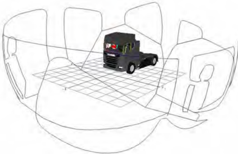
Figure 883. Combined direct and indirect FOV area projection for the Scania R N3
