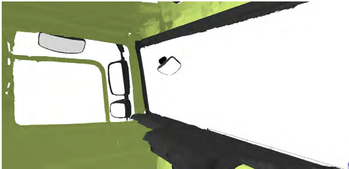
Figure 103. The view from the driver's eyes clearly shows the two cyclists are hidden from view.
