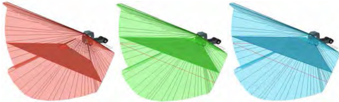
Figure 20. 3D Field of View Projection of the windscreen clipped to the ground plane (left), the ground plane +1738mm (middle) and the ground plane +1755mm (right)
