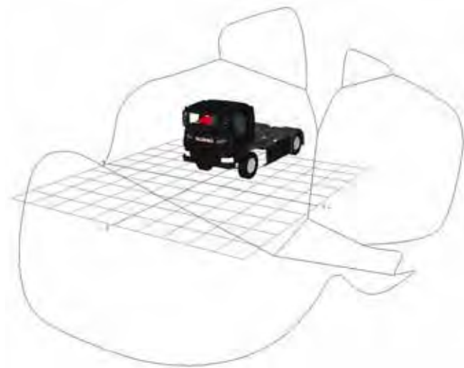
Figure 869. Combined indirect FOV area projection for the Scania P N3 / N3G
