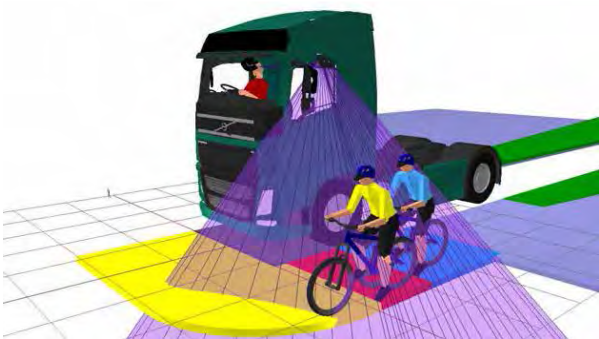
Figure 756. 3D volumetric projection showing the visibility of cyclist VRUs to the nearside of a vehicle with a 95 th %ile UK male driver using the Class V mirror adjusted for a 5 th %ile UK female
