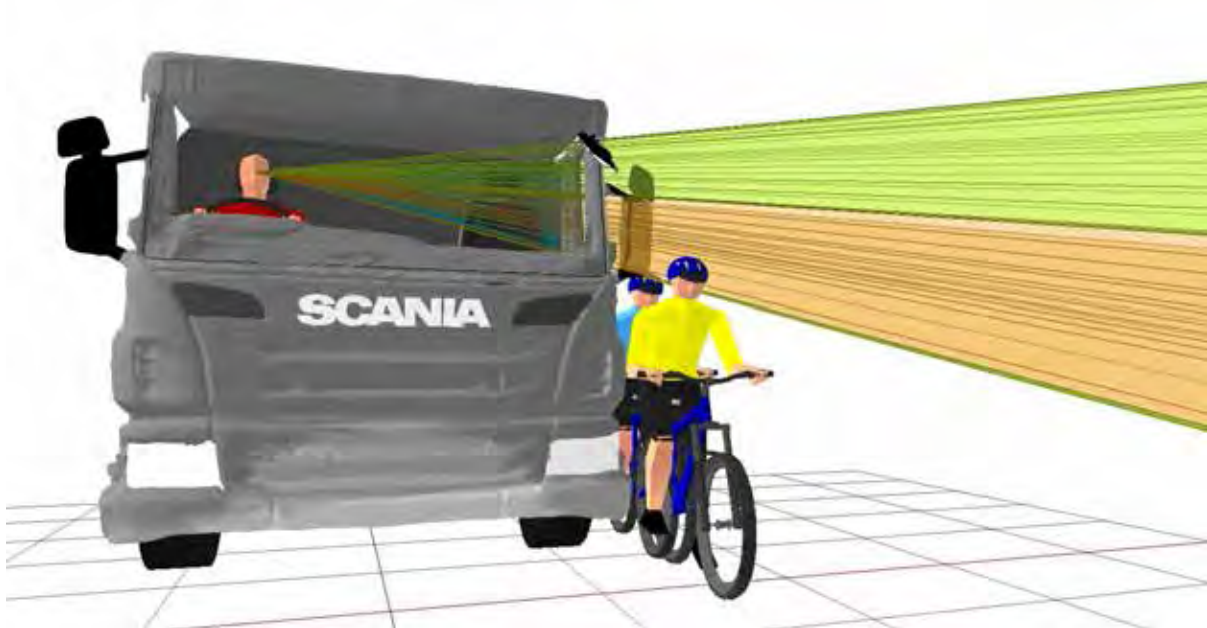
Figure 421. 3D view showing that the two human models can be seen through direct vision by the driver in the standardised driving posture
