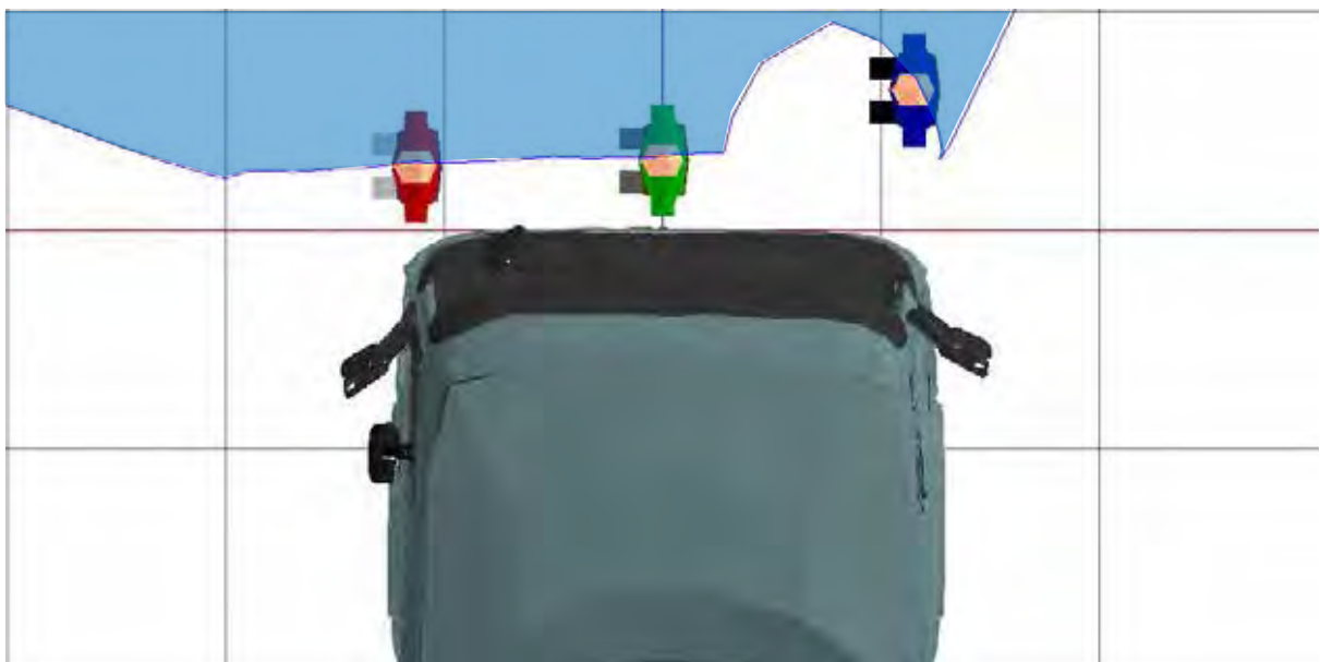
Figure 567. A plan view of the three human models that represent a pedestrian walking in front of a stationary vehicle and the projection of the windscreen at a height that equals the stature of a 50th%ile UK male pedestrian
