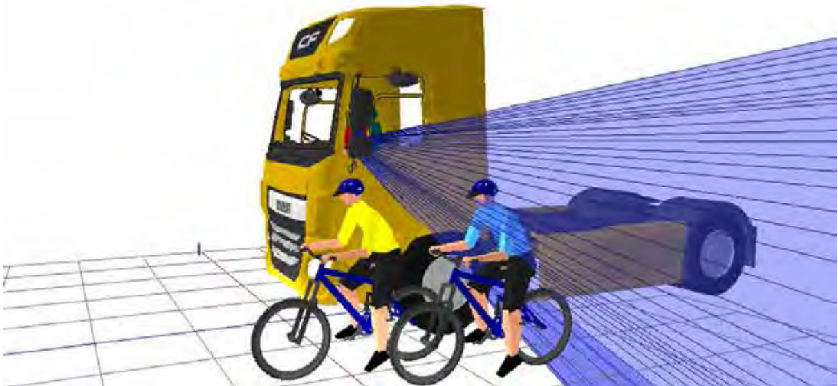
Figure 74. 3D view showing that the rear (blue) cyclist positioned to the nearside of the vehicle is visible in the projection of the Class IV mirror
