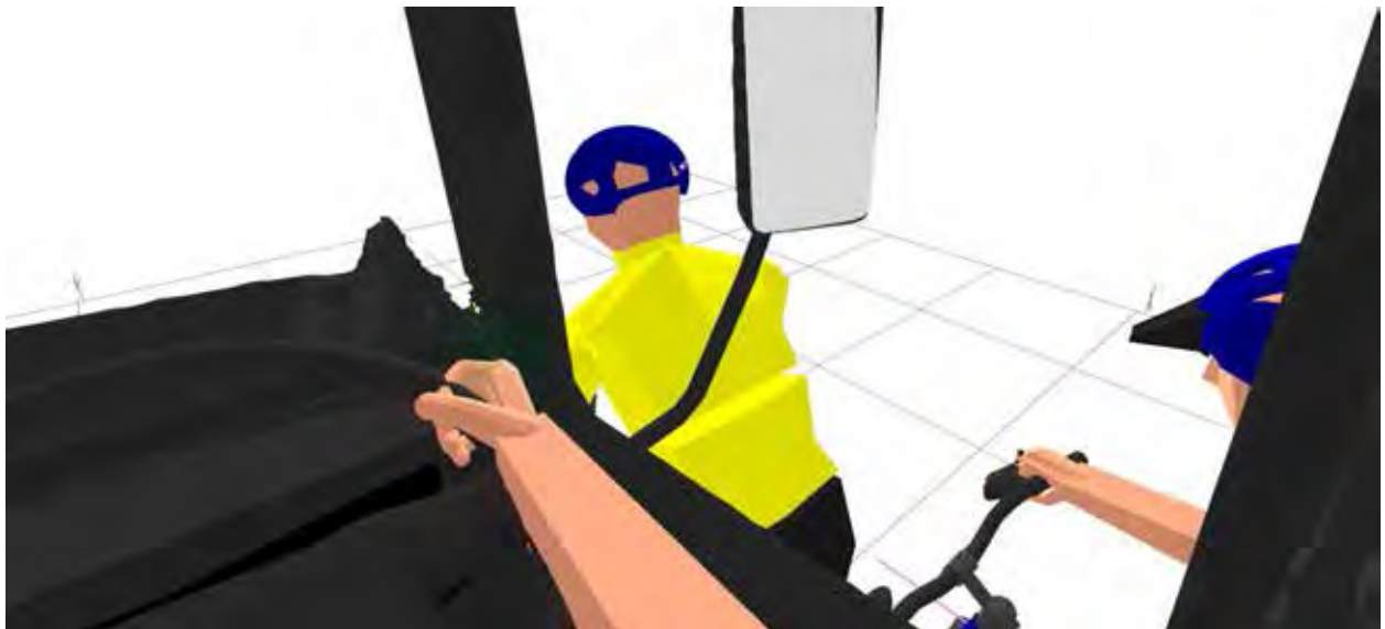
Figure 160. The view from the driver's eyes clearly shows the two cyclists are visible, even when positioned against the side of the vehicle.
