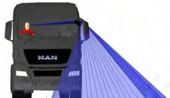
Figure 243. A front view of the Class V mirror projection for the MAN TGX N3
