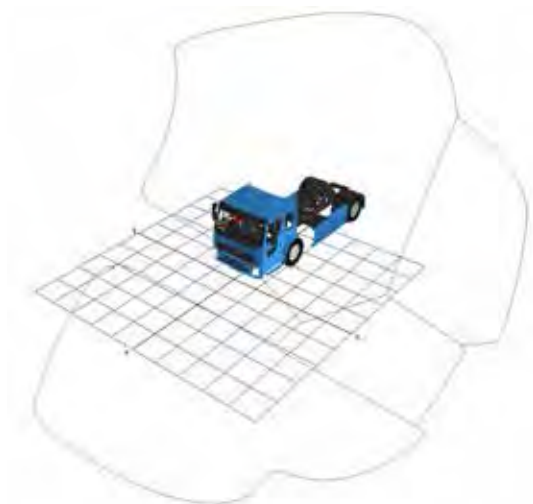
Figure 809. Combined indirect FOV area projection for the Volvo FE N3 LEC
