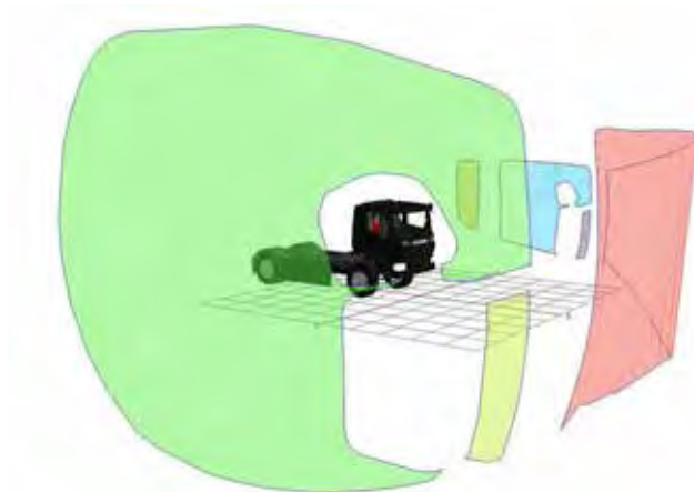
Figure 765. FOV area projection for the Scania P N3 / N3G
