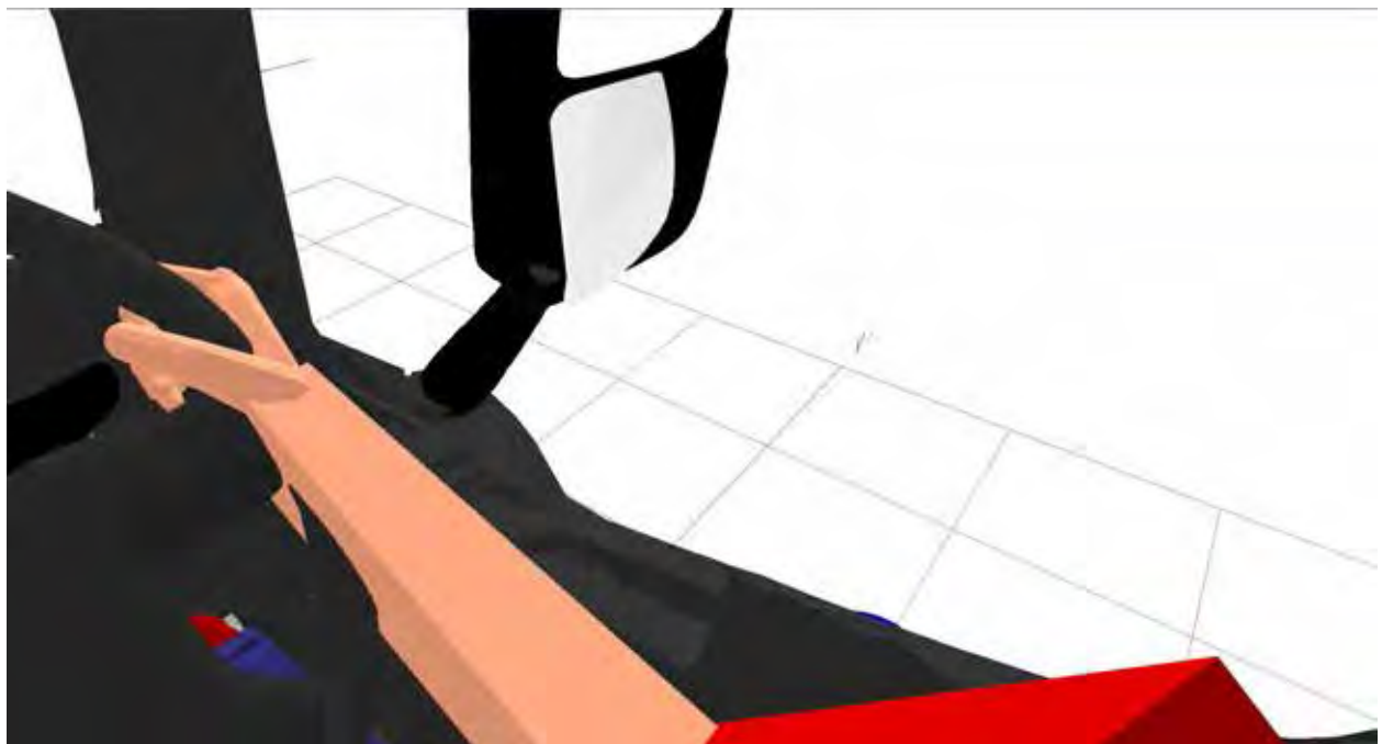
Figure 351. The view from the driver's eyes clearly shows the two cyclists are not visible
