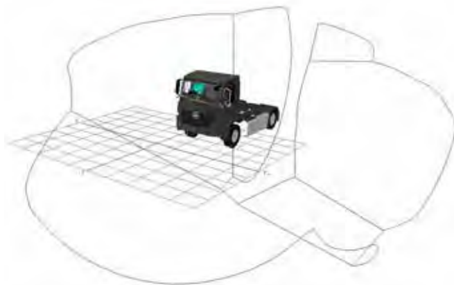
Figure 867. Combined indirect FOV area projection for the Mercedes Antos N3 / Arocs N3G / Actros N3
