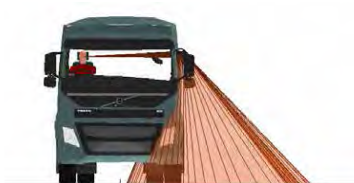
Figure 562. A front view of the Class V mirror projection for the Volvo FMX N3G
