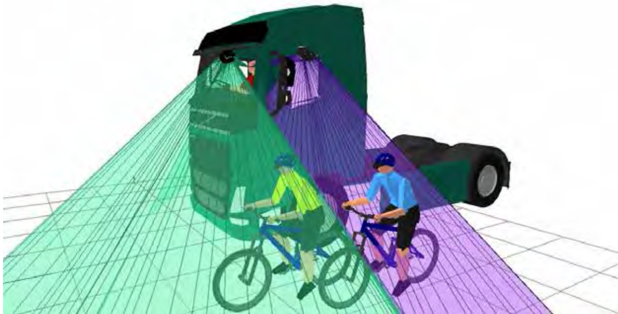
Figure 617. 3D view showing that both cyclists positioned to the nearside of the vehicle are visible in the projection of the Class V and / or Class VI mirrors
