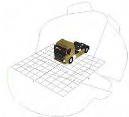
Figure 807. Combined indirect FOV area projection for the Volvo FM N3 / FMX N3G
