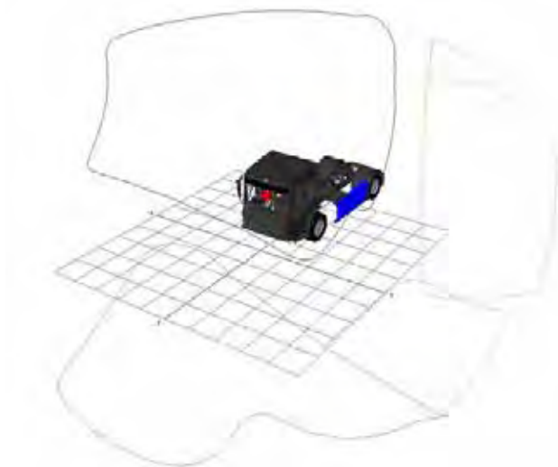
Figure 693. Combined indirect FOV area projection for the Dennis N3 LEC
