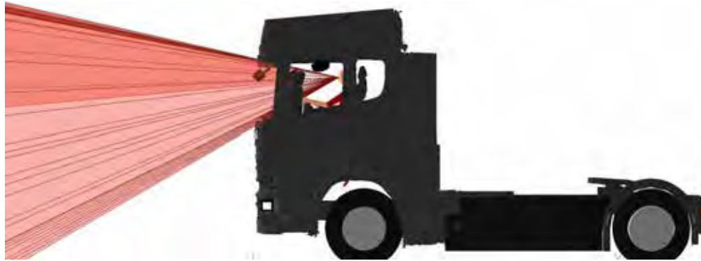
Figure 463. A side view of the windscreen aperture projection for the Scania R N3
