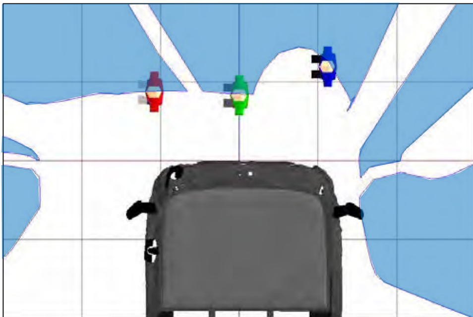
Figure 311. A plan view of the three human models that represent a pedestrian walking in front of a stationary vehicle and the projection of the windscreen at a height that equals the stature of a 50th%ile UK male pedestrian
