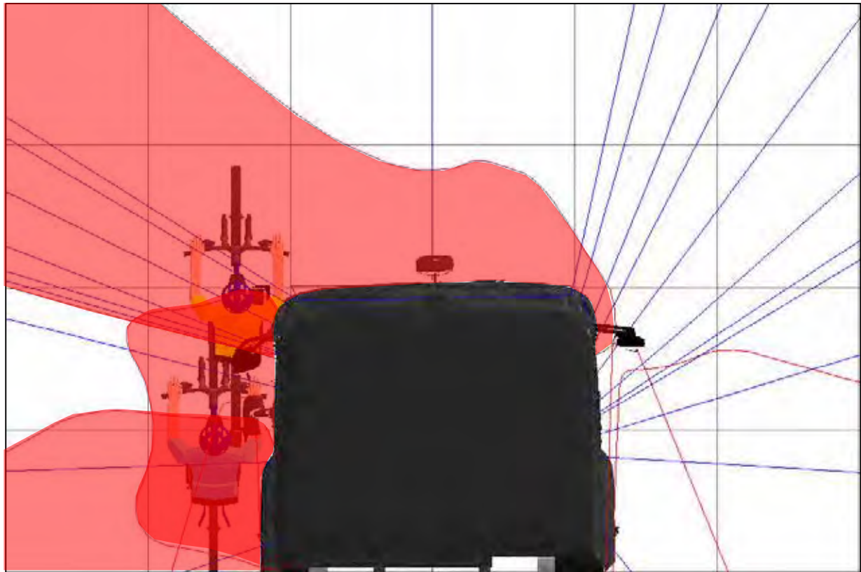
Figure 391. A plan view of the two human models that represent a cyclist moving up the inside of the vehicle and the projection of the Class IV, Class V and Class VI mirrors at a height that equals the stature of a 50th%ile UK male cyclist
