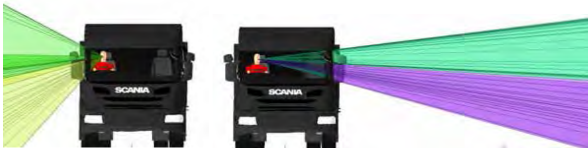
Figure 496. Frontal views of the off side and near side door window projections for the Scania N3 LEC
