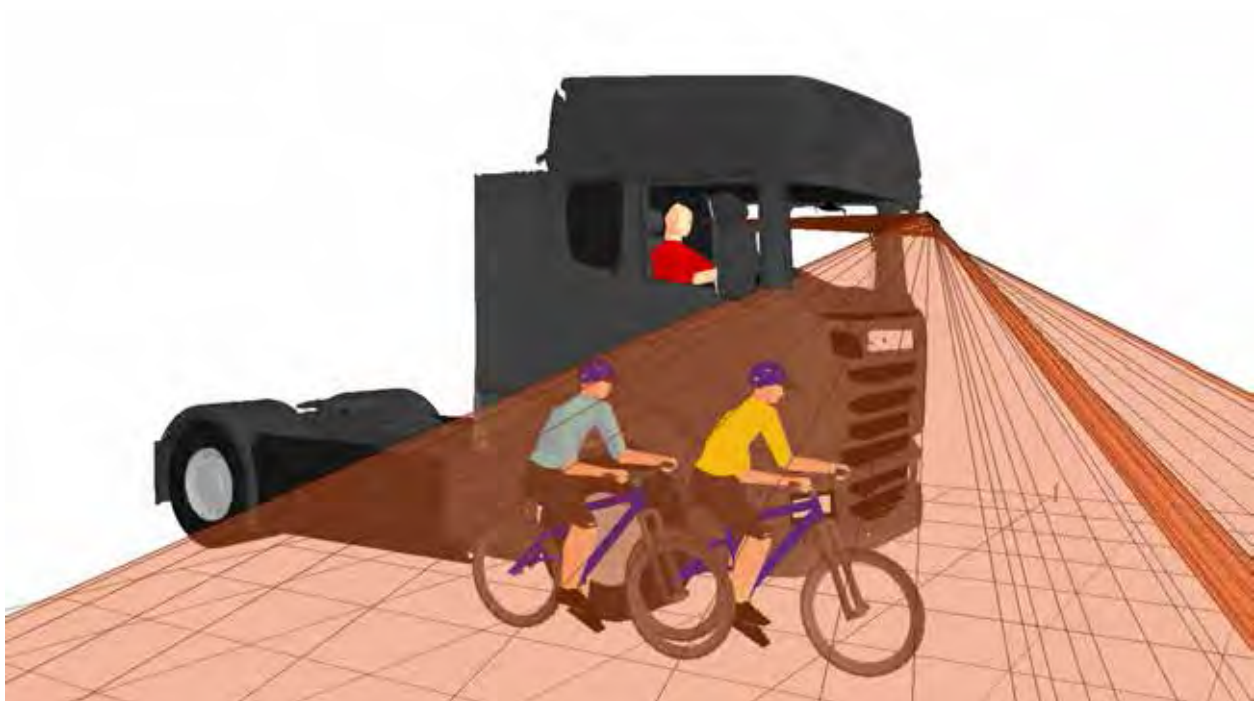
Figure 481. 3D view showing that the front (yellow) cyclist positioned to the offside of the vehicle is visible in the projection of the Class VI
