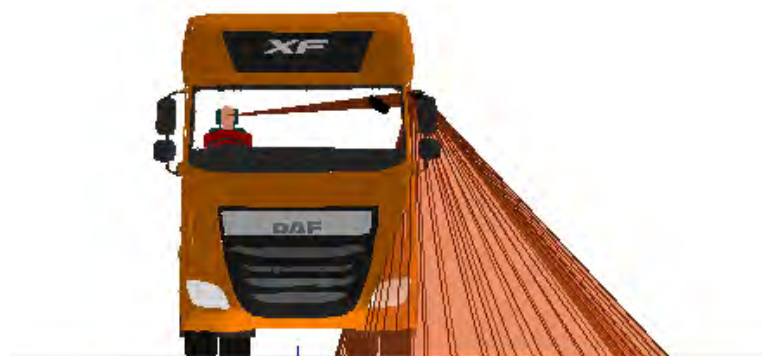
Figure 115. A front view of the Class V mirror projection for the DAF XF N3
