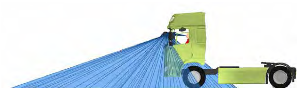
Figure 82. A side view of the Class VI mirror projection for the DAF CF N3G
