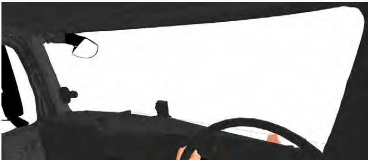
Figure 313. The view from the driver's eyes clearly shows the three pedestrians are hidden from view.
