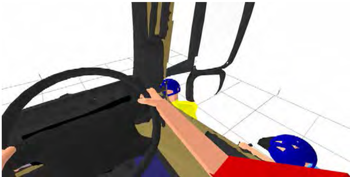
Figure 543. The view from the driver's eyes clearly shows the two cyclists are visible, even when positioned against the side of the vehicle.
