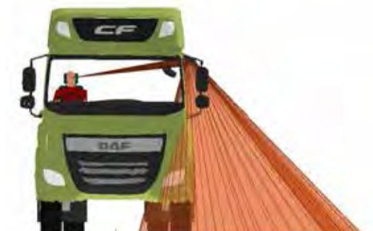
Figure 83. A front view of the Class V mirror projection for the DAF CF N3G
