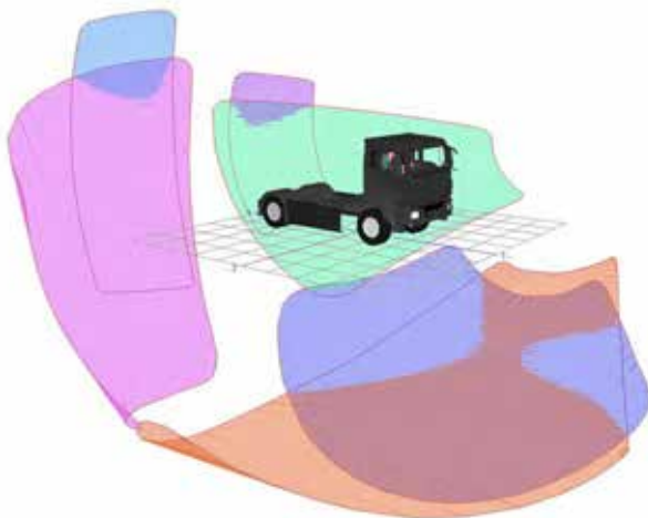
Figure 787. Indirect FOV area projection for the MAN TGS N3 / N3G
