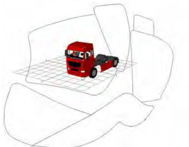
Figure 695. Combined indirect FOV area projection for the MAN TGX N3 / N3G
