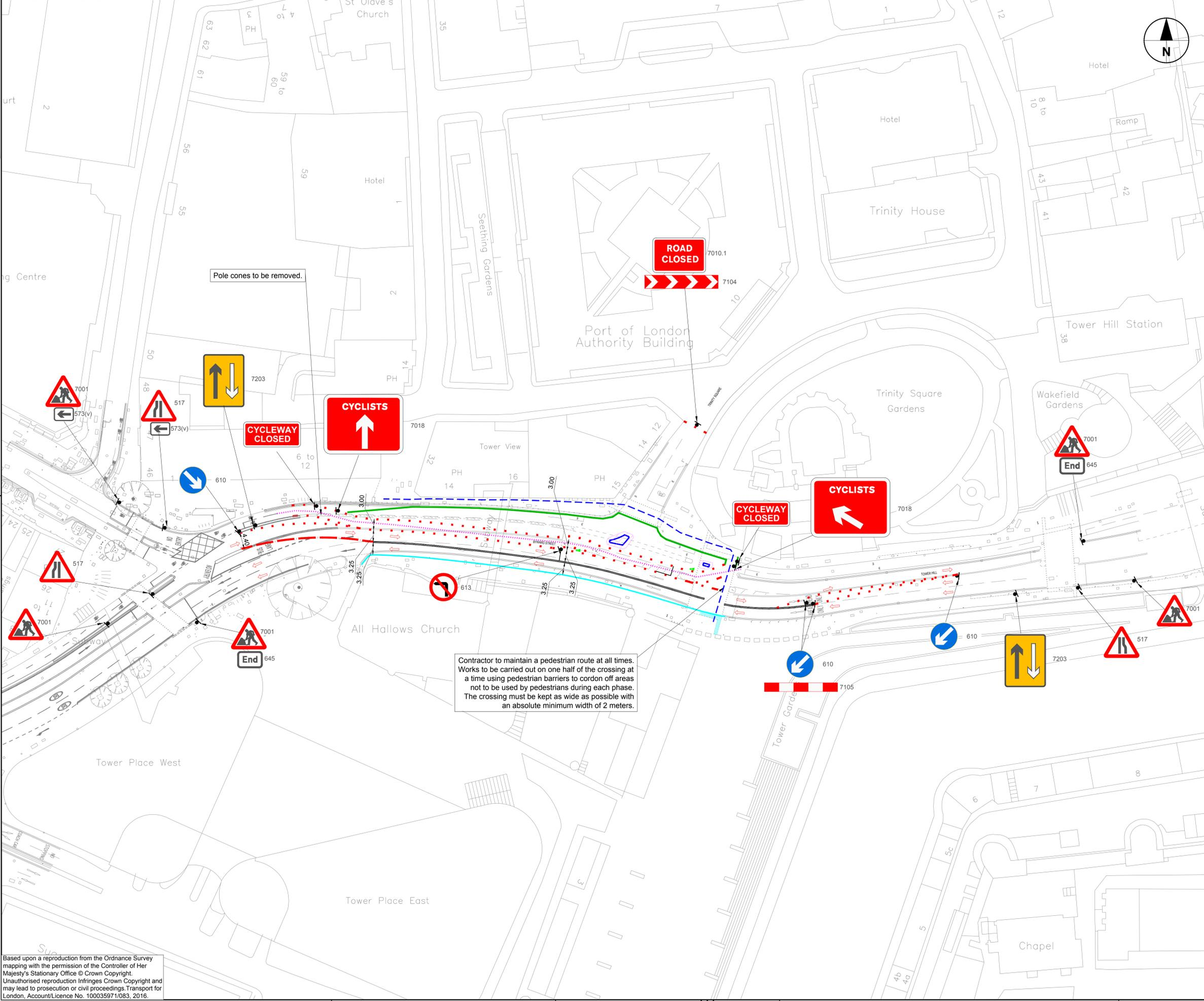
Contractor to maintain a pedestrian route at all times. Works to be carried out on one half of the crossing at a time using pedestrian barriers to cordon off areas not to be used by pedestrians during each phase. The crossing must be kept as wide as possible with an absolute minimum width of 2 meters.
