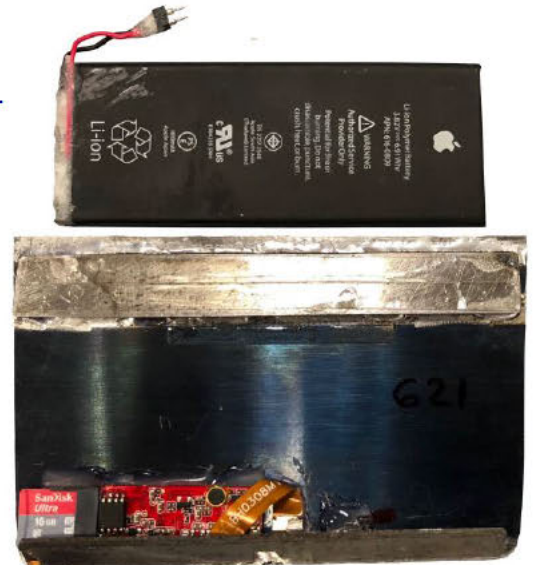
KENTISH TOWN DEVICE – COMPLETE WITH APPLE BATTERY AND 16GB SD MEMORY CARD
