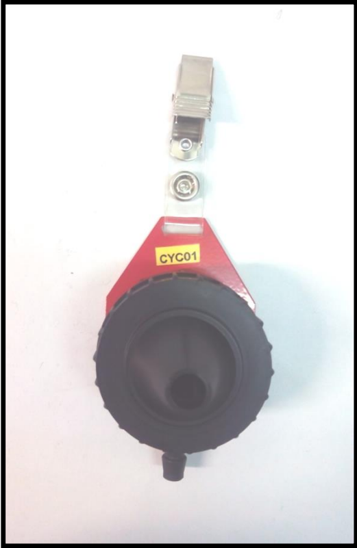
Figure 10. Cyclone Inhalable Sampler to monitor PM 2.5.
