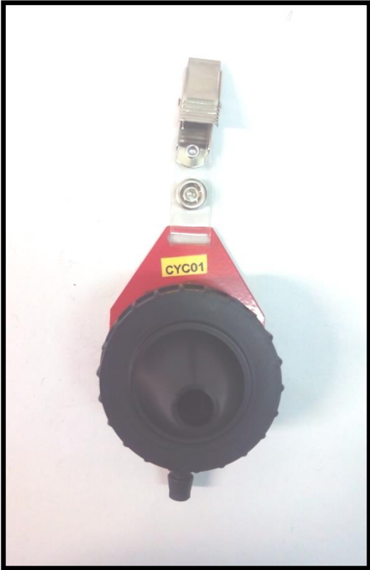
Figure 10. Cyclone Inhalable Sampler to monitor PM 2.5.
