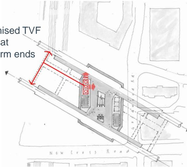
Increased tunnel ventilation duct length leads to increased fan sizes
