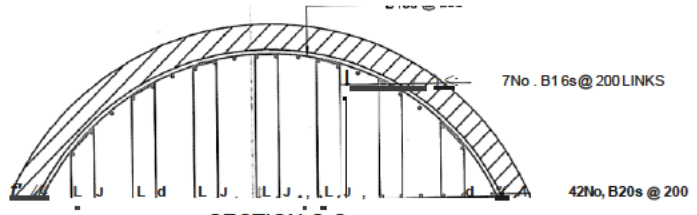
SECTION C-C REBAR DETAILS
