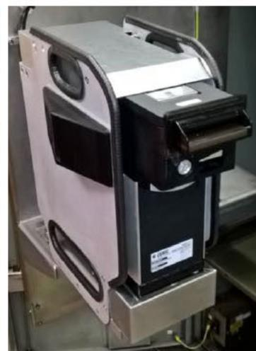
As a result a decision was taken to bring the unit into line with the other two units being trialed and to reconfigure the device to work as a Bank Note Acceptor and send all notes accepted to the note vault. This modification was undertaken during a site visit by a Cubic engineer on Tuesday 19 March.
