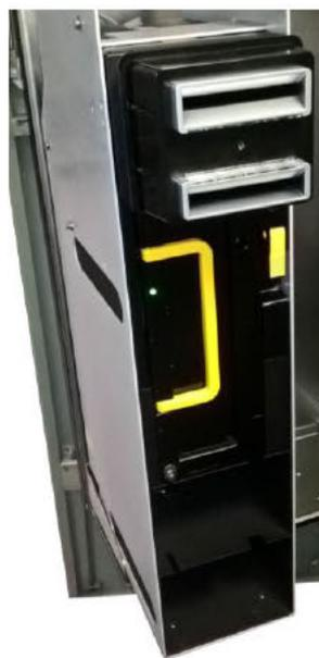
← The other note unit provided by CI tech and installed in MFM31 at Highbury & Islington, has also suffered some teething problems, with notes being jammed in the unit and some communications issues caused by the connection to the unit being damaged as the unit was rotated for servicing.
