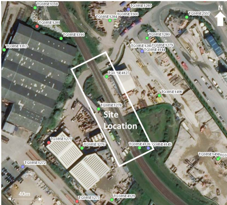
Figure 6-1 Borehole location plan
